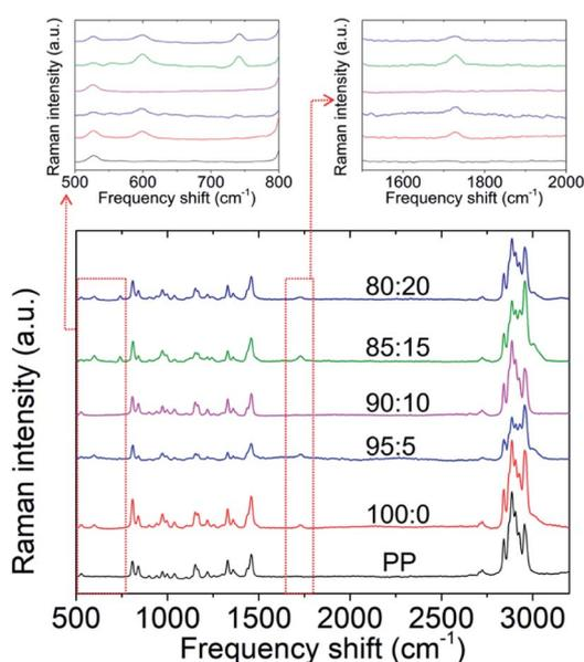
Fig. 1 Raman spectroscopy of the PMMA-based gel-polymer electrolyte (GPE).
