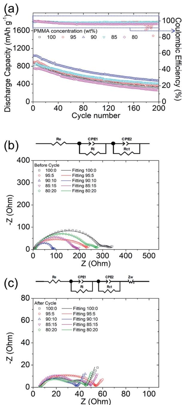
Fig. 2 Electrochemical analysis of lithium-sulfur cells with the polysulfide cathode and the PMMA-based GPEs with different PMMA : LiTFSI ratios: (a) cyclability for 200 cycles at a cycling rate of  $C/10$ ; and electrochemical impedance spectra (EIS) (b) before and (c) after cycling.
