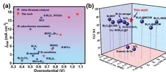
Fig. 3 (a) Literature overview of Bi-based electrocatalysts for the CO<sub>2</sub>-to-formate conversion. Overpotentials ( $\eta$ ) calculated using the equilibrium potential for CO<sub>2</sub>/HCOO<sup>-</sup>,  $E = -0.2$  V vs. RHE.<sup>34</sup> (b) Comparison of partial current density and FE of formate for the SU-101 NRs with those of previously reported Bi-based and other advanced catalysts at the applied potentials.
