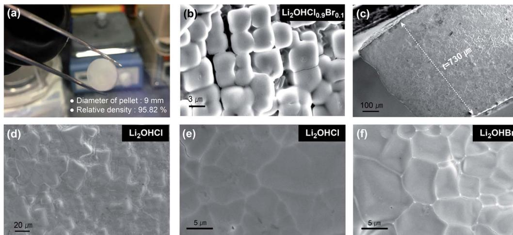
Fig. 3 (a) Digital photograph of  $\text{Li}_2\text{OHBr}$  antiperovskite solid electrolyte fabricated by melting and solidification. (b) The morphology of  $\text{Li}_2\text{OHCl}_{0.9}\text{Br}_{0.1}$  powder after melting and solidification. (c) Cross-sectional image of a  $\text{Li}_2\text{OHBr}$  pellet. Grain structure of a  $\text{Li}_2\text{OHCl}$  pellet at (d) low and (e) high magnifications. (f) Grain structure of an  $\text{Li}_2\text{OHBr}$  pellet at high magnification.
