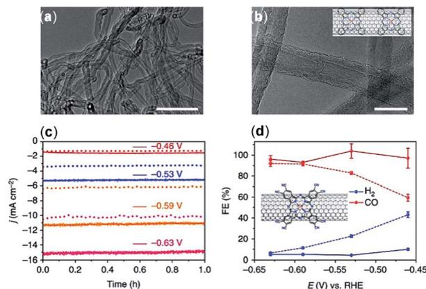
Fig. 3 (a and b) TEM images of the CoPc/CNT (6%) hybrid. Inset in (b) shows a schematic representation of the CoPc/CNT hybrid. (c) Representative chronoamperograms of CO<sub>2</sub> electroreduction catalyzed by the CoPc/CNT (2.5%) hybrid for 1 h at various potentials in 0.1 M KHCO<sub>3</sub> aqueous solution; (d) FE of reduction products at different potentials for CoPc–CN/CNT (solid line) and CoPc/CNT (dotted line).<sup>76</sup> Copyright 2017, Nature Publishing Group.
