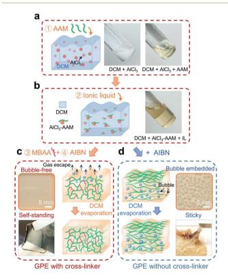
Fig. 1 Preparation schematic of the gel polymer electrolyte (GPE). (a) The complexation of the AAM monomer with AlCl<sub>3</sub> in DCM solvent. (b) Introducing abundant ionic liquid (IL). (c) The GPE polymerized with an MBAA cross-linker delivering a bubble-free and self-support membrane. (d) Typical fabrication showing a sticky GPE with bubbles.
