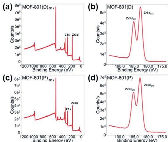
**Fig. 3** XPS spectra (a) and (b) for MOF-801(D) and (c) and (d) for MOF-801(P).
