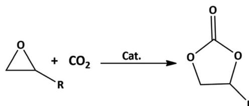
Fig. 1 Cycloaddition reaction of epoxide and CO<sub>2</sub> to form a five-membered cyclic carbonate (Cat. represents catalyst).
