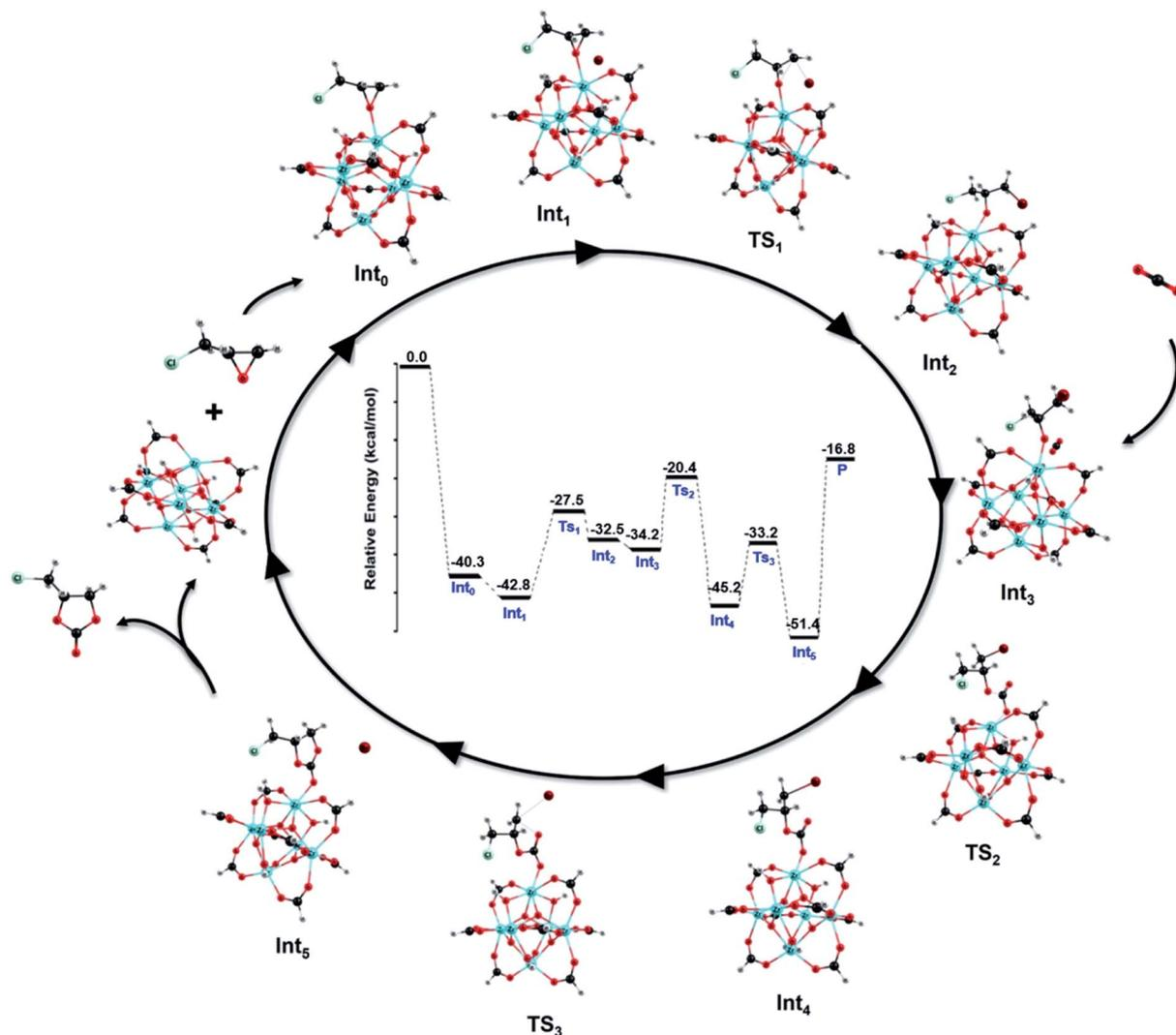
Fig. 8 Relative energy profile for the MOF-801/TBABr catalyzed cycloaddition reaction of CO<sub>2</sub> with ECH to form chloropropene carbonate and the DFT optimized structures of intermediates and transition states.
