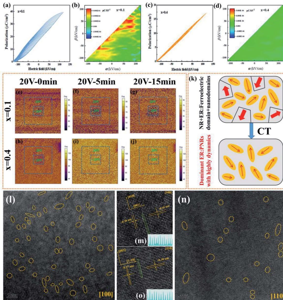
Fig. 5 FORC loops [(a) and (c)] and their evolution [(b) and (d)] for the incorporated ceramics; (e–j) PFM phase images after poling treatment and relaxation durations for  $x = 0.1$  and  $0.4$  samples; (k) schematic illustration of domain evolution resulting from CT incorporation. (l–o) HR-TEM images of domain morphology and lattice fringes along  $[100]_c$  and  $[110]_c$  for the  $x = 0.4$  ceramic.
