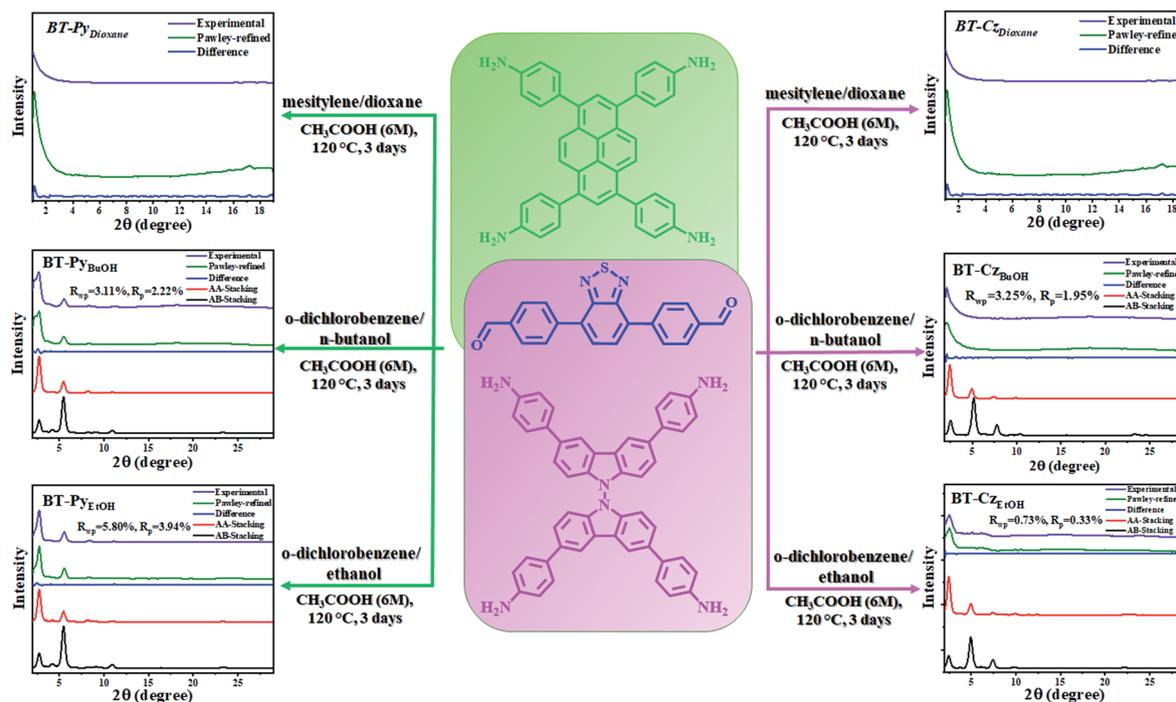
**Scheme 1** Schematic diagram of the structure and preparation of BT-Py<sub>Solvent</sub> and BT-Cz<sub>Solvent</sub> COFs in different solvents, and the experimentally observed PXRD patterns.
