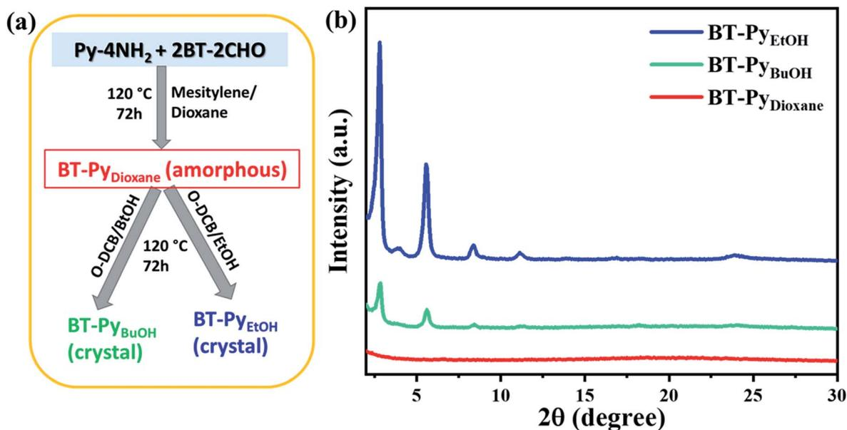
Fig. 7 (a) Schematic synthesis and (b) experimentally observed PXRD patterns of transforming amorphous material BT-Py<sub>Dioxane</sub> COF into crystalline BT-Py<sub>BuOH</sub> COF and BT-Py<sub>EtOH</sub> COF.
