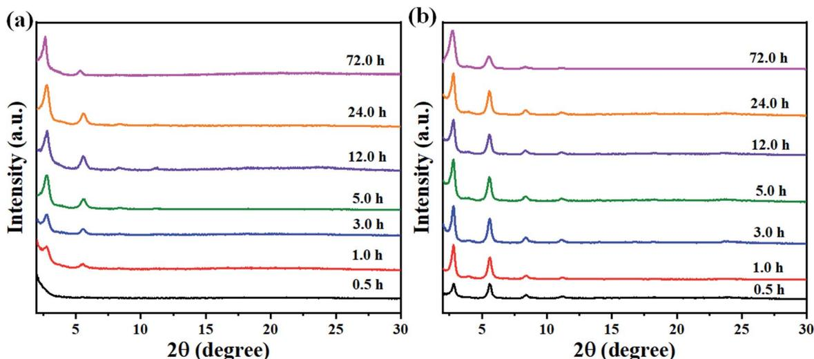
Fig. 6 Experimentally observed PXRD patterns of (a) BT-Py<sub>BuOH</sub> COF and (b) BT-Cz<sub>EtOH</sub> COF at different reaction times.
