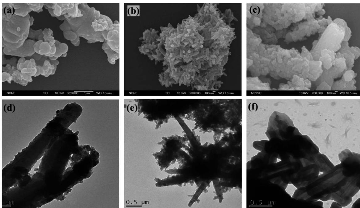
Fig. 3 FE-SEM images of (a) BT-Py<sub>Dioxane</sub>, (b) BT-Py<sub>BuOH</sub>, and (c) BT-Py<sub>EtOH</sub>. TEM images of (d) BT-Py<sub>Dioxane</sub>, (e) BT-Py<sub>BuOH</sub>, and (f) BT-Py<sub>EtOH</sub>.
