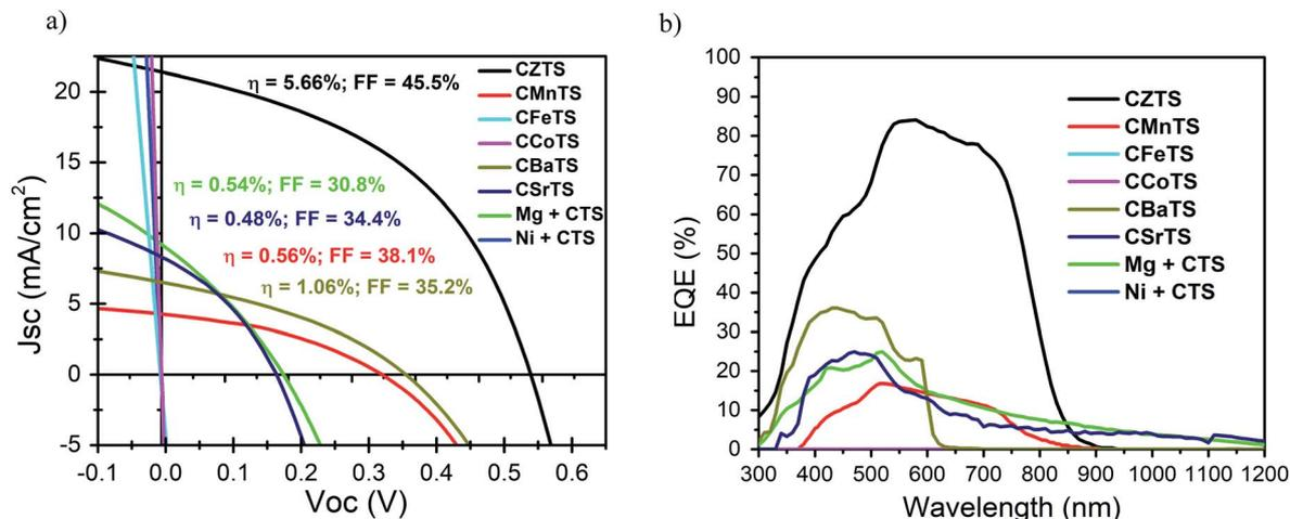
Fig. 4 (a)  $J$ - $V$  curve for the "champion" cell from each of the CXTS films. (b) External quantum efficiency for the CXTS solar cells with their respective extracted band gap and  $J_{sc}$ . Each CXTS film (represented by different colors) has two EQE responses; the solid line represents the post annealed film response and dashed line represents the response for the film without post annealing.
