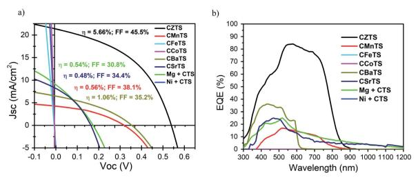
Fig. 4 (a) J-V curve for the "champion" cell from each of the CXTS films. (b) External quantum efficiency for the CXTS solar cells with their respective extracted band gap and Jsc. Each CXTS film (represented by different colors) has two EQE responses; the solid line represents the post annealed film response and dashed line represents the response for the film without post annealing
