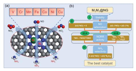
Fig. 1 (a) The atomic structure of M1M2@NG DACs (M1/M2 = V, Cr, Mn, Fe, Co, Ni, and Cu). (b) The optimized strategy for screening NORR electrocatalysts including four stepwise selection principles. The third criterion consists of "two steps of key hydrogenation process".
