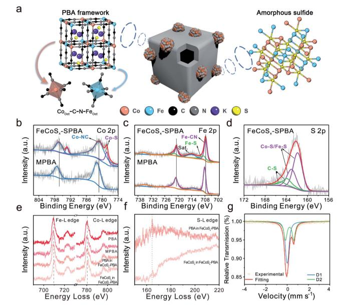
Fig. 2 (a) Schematic diagrams of FeCoS<sub>x</sub>-PBA. (b) Co 2p and (c) Fe 2p XPS spectra of FeCoS<sub>x</sub>-PBA and MPBA. (d) S 2p XPS spectra of FeCoS<sub>x</sub>-PBA. (e) Co L<sub>2.3</sub> and Fe L<sub>2.3</sub> edge EELS spectra of PBA, MPBA, and FeCoS<sub>x</sub>-PBA. (f) S L<sub>2.3</sub> edge EELS spectra of FeCoS<sub>x</sub>-PBA. (g) Mössbauer spectrum pattern of FeCoS<sub>x</sub>-PBA
