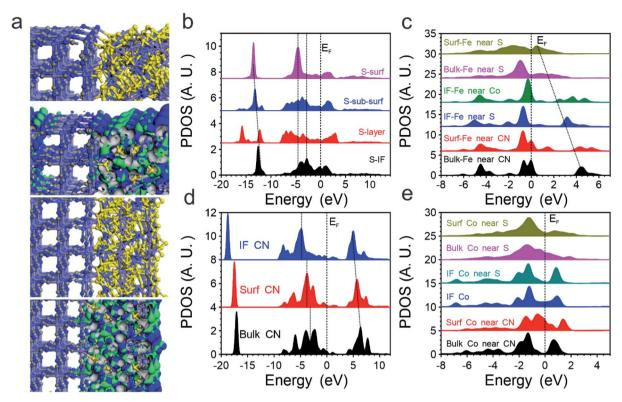
Fig. 3 The electronic structures of FeCoS<sub>x</sub>-PBA. (a) Structural configurations and real spatial 3D orbital contour plots of two different FeCoS<sub>x</sub>-PBA systems. (b) Site-dependent PDOSs of S in FeCoS<sub>x</sub>-PBA. (c) Site-dependent PDOSs of Fe in FeCoS<sub>x</sub>-PBA. (d) Site-dependent PDOSs of Co in FeCoS<sub>x</sub>-PBA. (e) Site-dependent PDOSs of -CN in FeCoS<sub>x</sub>-PBA.
