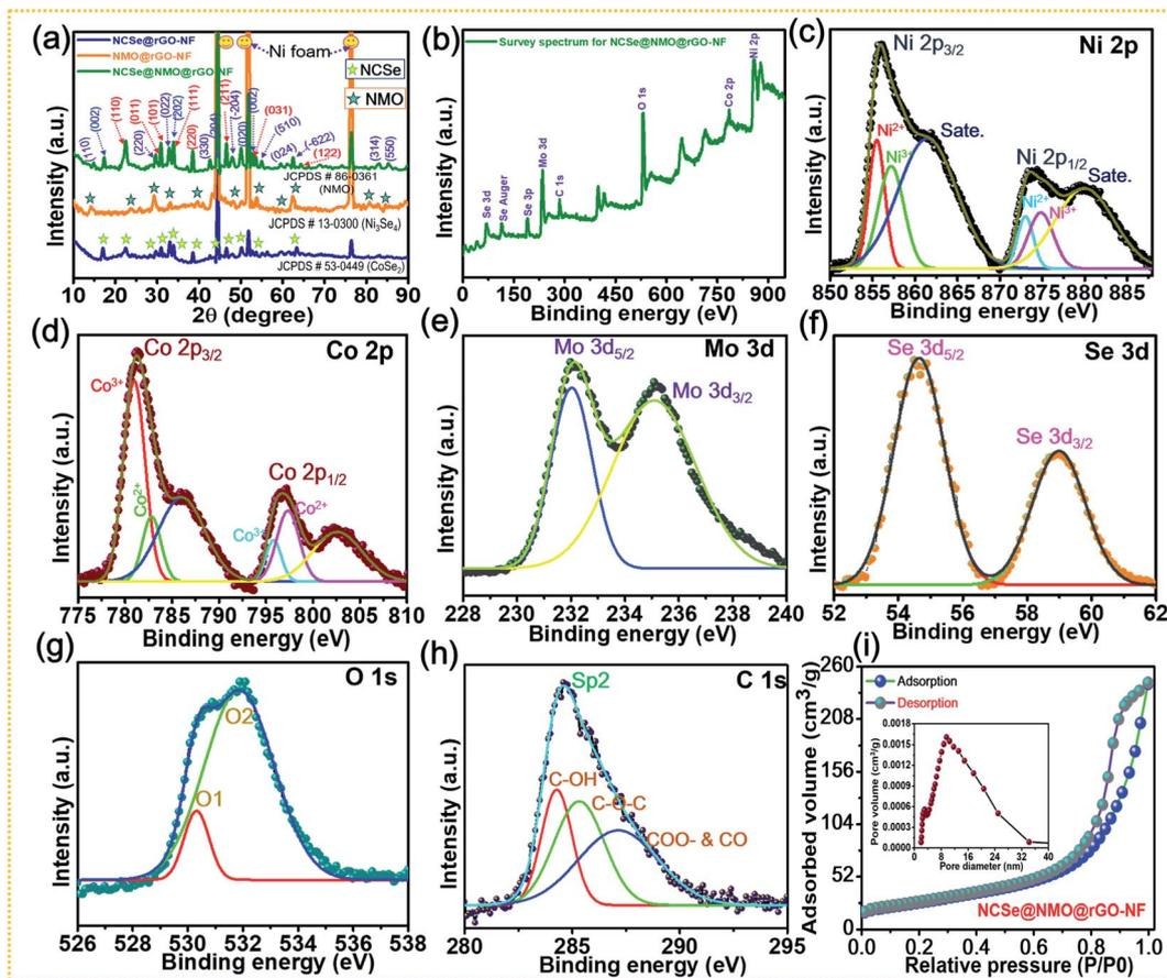
Fig. 4 (a) XRD patterns of NCSe@rGO-NF, NMO@rGO-NF, and NCSe@NMO@rGO-NF. (b) XPS survey spectra of NCSe@NMO@rGO-NF. Core-level spectra of various elements: (c) Ni 2p, (d) Co 2p, (e) Mo 3d, (f) Se 3d, (g) O 1s, (h) C 1s in NCSe@NMO@rGO-NF. (i) BET analysis showing a typical  $N_2$  adsorption-desorption isotherm and pore size distribution curve (inset) of the NCSe@NMO@rGO-NF core-shell structure.
