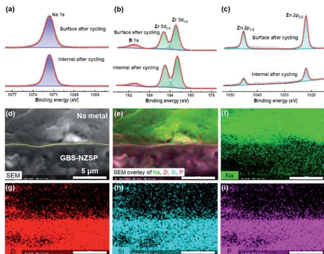
Fig. 4 Interface analysis of GBS-NZSP ( $x = 0.2$ ) after Na plating/stripping cycles. XPS spectra of (a) Na 1s, (b) Zr 3d and B 1s, (c) Zn 2p with the comparison between the upper surface and the internal cross section. (d) SEM image and (e–i) corresponding elemental mapping images of the cross-sectional Na-metal capped GBS-NZSP.
