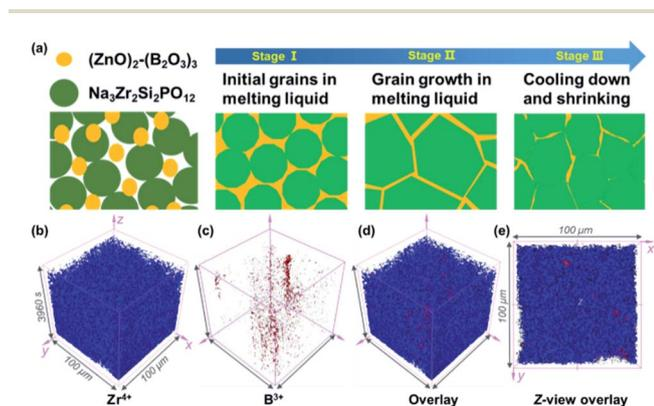
Fig. 1 (a) Schematic of the liquid-phase sintering of GBS-NZSP using the ZBO additive and (b–e) the 3D rendered model of the selected sample with ZBO molar ratio  $x = 0.2$  according to the depth profile by ToF-SIMS.
