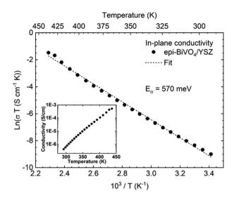
Fig. 4 Temperature-dependent in-plane conductivity of epi-BiVO<sub>4</sub>/YSZ. Conductivity,  $\sigma$ , plotted as  $\ln(\sigma T)$  vs.  $10^3/T$ . The dashed line represents the fit to eqn (1), yielding a charge transport activation energy,  $E_{\sigma}$ , of 570 meV. In the inset, the conductivity is plotted against the temperature in a semi-log plot.
