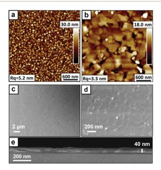
Fig. 2 Morphological analysis of BiVO<sub>4</sub>/YSZ before and after the solidstate transformation. AFM topography images of (a) poly-BiVO<sub>4</sub>/YSZ starting material and (b) epi-BiVO<sub>4</sub>/YSZ after annealing at 650  $^{\circ}$ C. (c and d) Top-view SEM and (e) cross-sectional SEM images of epi-BiVO<sub>4</sub>/YSZ.
