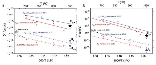
Fig. 3 Diffusivity (a) and surface exchange coefficient (b) for nanocrystalline LSM measured by APT and compared to literature values (for stoichiometric and B-site deficient (LSM<sub>0.85</sub>) materials).<sup>13,14,29</sup> Values from Saranya et al. 2015 (ref. 14) have been updated using the FEM model introduced by the authors in Saranya et al. 2018 (ref. 18). The error bars are calculated from the sensitivity analysis described in ESI Note 2.†
