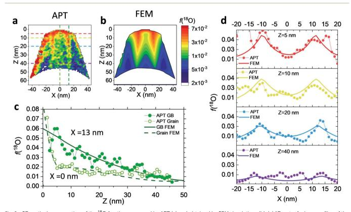
Fig. 2 Devertical cross section of the <sup>18</sup>O fraction measured by APT (a) and obtained by FEM simulations (b). (c) 1D out-of-plane profiles of the isotope fraction obtained along a GB and along the grain bulk of the LSM tip, as measured by IE-APT and calculated in the FEM simulation. (d) 1D horizontal <sup>18</sup>O fraction measured at different distances from the sample's surface. The vertical and horizontal 1D profiles shown in (c) and (d) are depicted in a as dashed lines.
