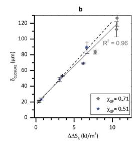
Fig. 3 Closure displacement relation to released entropy in wide range of healing temperature for two specific systems ( $\chi_{SF} = 0.71$  and 0.51). (a)  $\Delta S_R$  dependence on  $T_{retraction}$ . (b)  $\delta_{CLOSURE}$  dependence on  $\Delta S_R$ .
