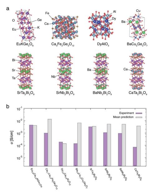
Fig. 18 (a) Graphics of the unit cells of the host materials of oxygen-ion conductors; (b) experimental and predicted values for the oxygen-ion conductivities  $\sigma$  at 700 °C. Reprinted with permission from ref. 154 (2020) Nature Publisher.
