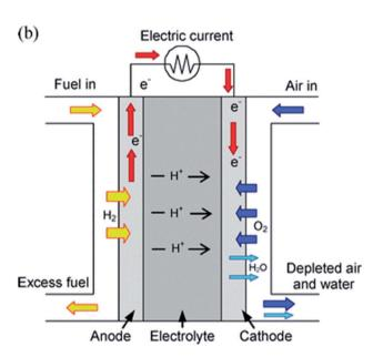
Fig. 1 Schematic diagram of the processes taking place in a SOFC during operation with a (a) oxide-ion conducting and (b) proton conducting electrolyte, respectively. Copyright (2010) Royal Society of Chemistry.
