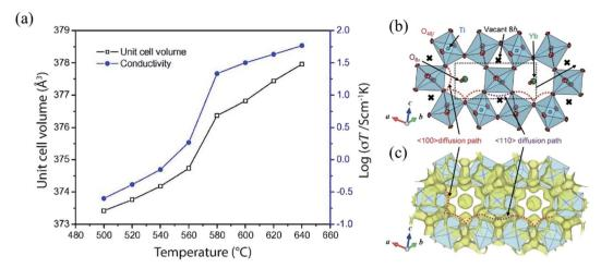
Fig. 11 (a) The correlation between the unit cell volume and the bulk conductivity of  $La_2Mo_2O_9$ . Adapted from ref. 86. Copyright (2011) Elsevier Publisher. (b) A part of the refined crystal structure and (c) equidensity surface of the MEM neutron scattering length density distribution of  $Yb_2Ti_2O_7$  at 1173 K at 0.002 fm  $A^{-3}$ . Reprinted with permission from ref. 90. Copyright (2018) JCS-Japan.
