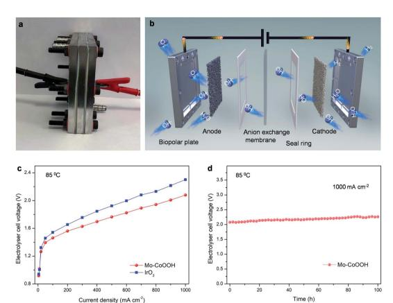
Fig. 4 Performance of Mo-CoOOH catalysts in practical electrolyser systems. (a) Photograph of an alkaline anion exchange membrane electrolyzer device. (b) Schematic illustration of the electrolyser structure. (c) Polarization curves for water electrolysis using Mo-CoOOH or commercial precious IrO2 as the anode catalyst and 20% Pt/C as the cathode catalyst. (d) Durability of the electrolyser at a constant current density of 1000 mA cm<sup>-2</sup> for 100 h at 85 °C.
