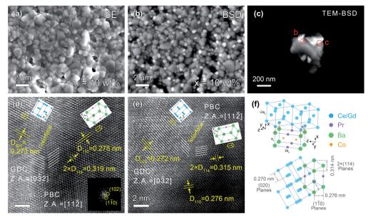
Fig. 2 SEM-SE (a) and SEM-BSD (b) surface images of PBC-10 wt% GDC pellet at the same location, respectively. (c) TEM-BSD image of PBC-10 wt% GDC composite; (d and e) HR-TEM images of PBC and GDC phase interface highlighting the lattice planes and orientations. (f) Schematic of crystal orientation relationship of PBC and GDC phases
