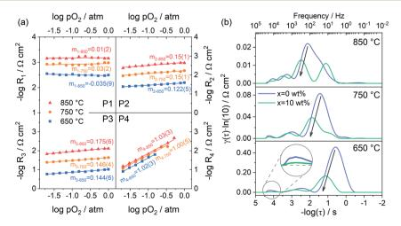
Fig. 7 (a) Polarization resistance as a function of oxygen partial pressure at different temperatures for sample PBC-10 wt% GDC. (b) DRT spectra of PBC-xGDC (x = 0 and 10 wt%) composite electrode measured in air.
