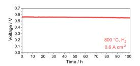
Fig. 10 Durability test in constant current density mode with hydrogen as fuel at  $800\,^{\circ}\text{C}$ .
