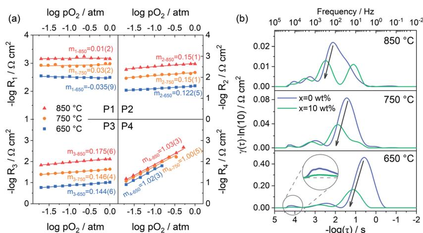
Fig. 7 (a) Polarization resistance as a function of oxygen partial pressure at different temperatures for sample PBC–10 wt% GDC. (b) DRT spectra of PBC– $x$ GDC ( $x = 0$  and 10 wt%) composite electrode measured in air.
