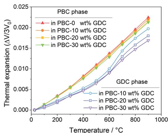
Fig. 3 Temperature-dependent linear thermal expansion of PBC-*x*GDC (*x* = 0, 10, 20 and 30 wt%) samples obtained from Rietveld refinement results.
