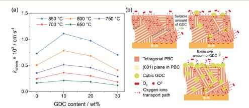
Fig. 5 (a)  $k_{\text{chem}}$  versus GDC mass fraction at various temperatures for PBC-xGDC (x = 0, 10, 20 and 30 wt%). (b) Schematics of the oxygen transport path in the composite bar with varying contents of GDC.
