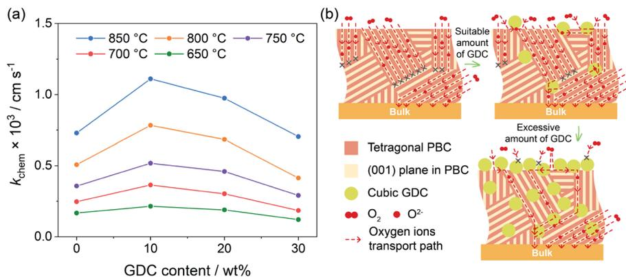
Fig. 5 (a)  $k_{\text{chem}}$  versus GDC mass fraction at various temperatures for PBC-xGDC ( $x = 0, 10, 20$  and  $30$  wt%). (b) Schematics of the oxygen transport path in the composite bar with varying contents of GDC.
