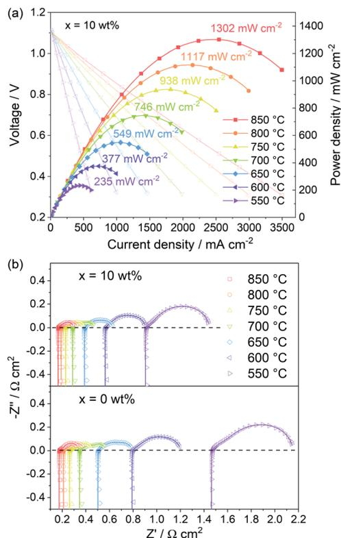
Fig. 9 (a)  $I$ - $V$  and power density curves of the electrolyte-supported cell with PBC-10 wt% GDC composite cathode at different temperatures fed with humidified  $H_2$ . (b) Impedance spectra of the cell with PBC-10 wt% GDC and pure PBC as cathode at different temperatures. The scatters are original data, and the lines are fitting data.
