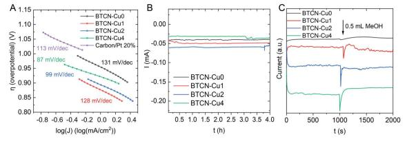
Fig. 6 (A) Calculated Tafel slopes of BTCN-Cu0, BTCN-Cu1, BTCN-Cu2, BTCN-Cu4 and Pt/C, (B) chronoamperometry curves at 0.15 V vs. Ag/ AqCl (sat. KCl) over 4 hours and (C) chronoamperometry curves at 0.15 V vs. Aq/AqCl (sat. KCl) after the injection of 0.5 mL MeOH.
