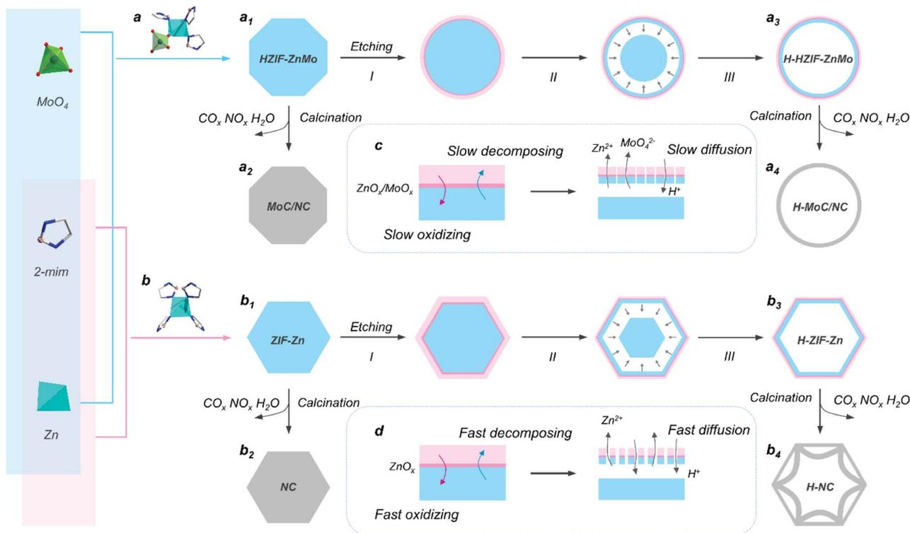
Fig. 1 (a) and (b) The crystalline structure of HZIF-ZnMo and ZIF-Zn. ( $a_1$ – $a_4$ ) The schematic morphologies for HZIF-ZnMo, MoC/NC, H-HZIF-ZnMo and H-MoC/NC. ( $b_1$ – $b_4$ ) The schematic morphologies for ZIF-Zn, NC, H-ZIF-Zn and H-NC; (c and d) the chemical etching process schemes for HZIF-ZnMo and ZIF-Zn.
