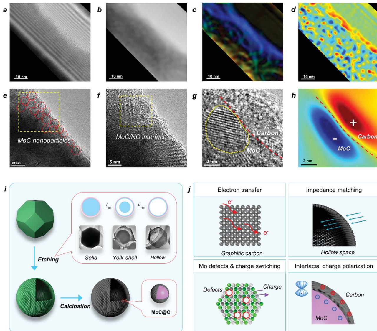
Fig. 5 (a) Hologram. (b) Reconstructed phase image. (c) Electric-field map. (d) Charge density map. (e) HR-TEM images. (f and g) MoC/NC hetero-interface. (h) Charge distribution on the MoC(-)/carbon(+) interface. (i) Two-step synthetic route and chemical etching mechanism (insert). (j) Illustration schemes of four electromagnetic wave attenuation mechanism.
