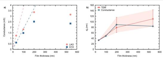
Fig. 6 (a) Measured equilibrium conductance by Van-der-Pauw measurements at 375 °C in high pO<sub>2</sub>. Dashed lines are extrapolations of the expected conductance of a fully dense layer. (b) Thickness of the dense bottom layer,  $d_d$ , for L2NO4/LAO samples, estimated from conductance measurements assuming constant conductivity and via TEM measurements. Filled area indicates observed variations of the dense layer thickness by TEM, e.g. minimum and maximum values.
