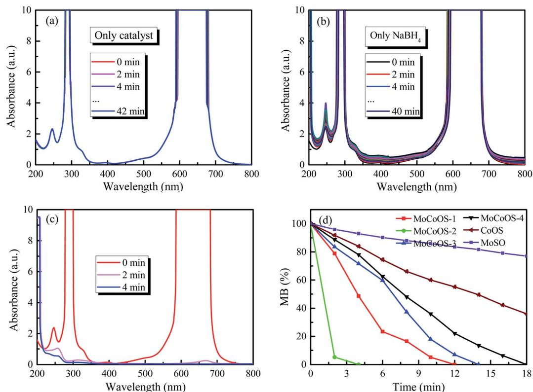
Fig. 10 (a) Reaction of MB with only MoCoOS-2. (b) Reaction of MB with only NaBH<sub>4</sub>. (c) Reduction of MB with MoCoOS-2 and NaBH<sub>4</sub>. (d) Reduction of MB with Mo(S,O), Co(O,S), and MoCoOS catalysts in the presence of NaBH<sub>4</sub>.
