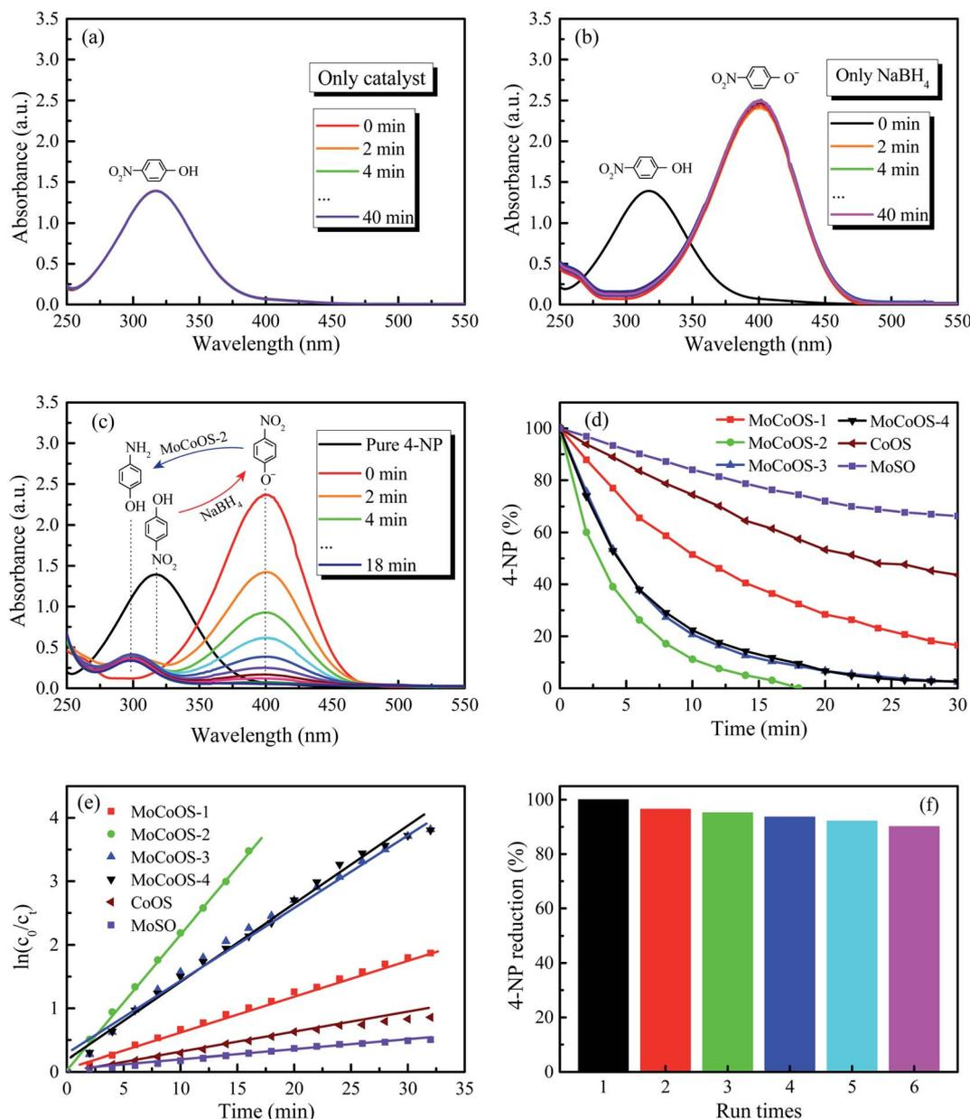
Fig. 8 (a) Reaction of 4-NP with MoCoOS-2. (b) Reaction of 4-NP with NaBH<sub>4</sub>. (c) Reduction of 4-NP with MoCoOS-2 and NaBH<sub>4</sub>. (d) Reduction of 4-NP with Mo(S,O), Co(O,S), and MoCoOS catalysts in the presence of NaBH<sub>4</sub>. (e) The first order reaction rate curves of 4-NP. (f) Catalytic reduction efficiency after cycles of reactions.
