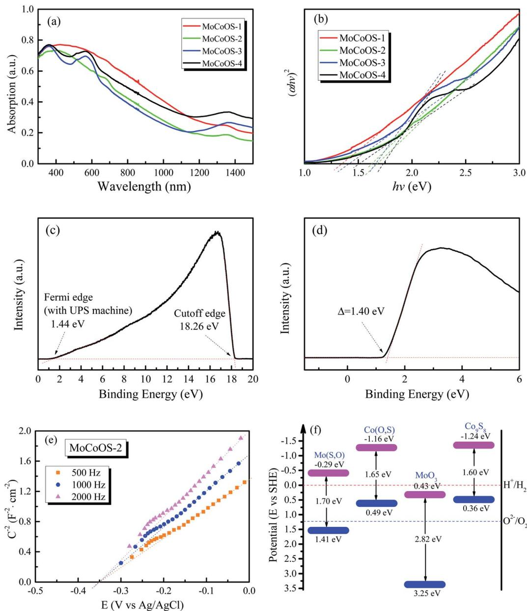
Fig. 5 (a) UV-vis absorption spectra of MoCoOS. (b) The  $(\alpha hv)^2 - hv$  plots from the ultraviolet absorption spectra. (c) UPS spectrum of MoCoOS-2. (d) XPS-VB spectrum of MoCoOS-2. (e) Mott-Schottky curve of MoCoOS-2. (f) Band structure alignment of catalysts.
