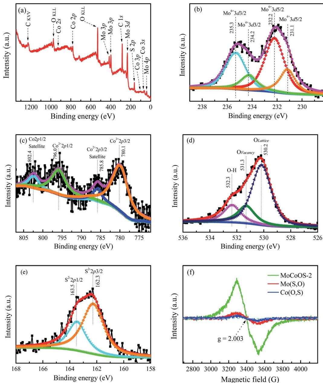
Fig. 1 (a) Survey spectrum and high resolution (b) Mo 3d, (c) Co 2p, (d) O 1s, and (e) S 2p XPS spectra of the MoCoOS-2 catalyst. (f) EPR spectra of the MoCoOS-2 catalyst, Mo(S,O), and Co(O,S).
