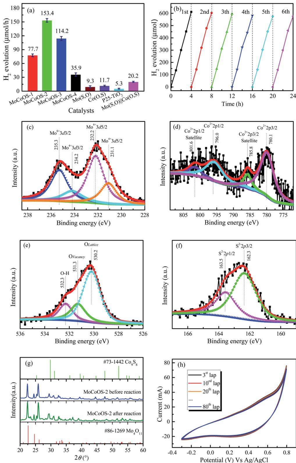
Fig. 7 (a) Hydrogen production of MoCoOS, Mo(S,O), Co(O,S), Mo(S,O)||Co(O,S) and P25-TiO<sub>2</sub> catalysts. (b) Recycling hydrogen production reaction performance of MoCoOS-2. (c-f) XPS spectra of MoCoOS-2 after the hydrogen evolution reaction. (g) XRD patterns of MoCoOS-2 before and after the hydrogen evolution reaction. (h) Cyclic voltammetry of MoCoOS-2 for 80 cycles.
