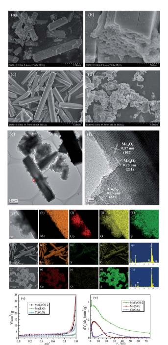
Fig. 4 (a and b) SEM images of MoCoOS-2. SEM images of (c) Mo(S,O) and (d) Co(O,S). (e) TEM and (f) HR-TEM images of MoCoOS-2. (g-k) EDX element distribution mapping images of Mo, Co, O, and S for MoCoOS-2. (1-p) EDX element distribution mapping images of Mo, O, and S for Mo(S,O). (q-u) EDX element distribution mapping images of Co, O, and S for Co(O,S). (v) Nitrogen adsorption-desorption isotherm and (w) the pore size distribution curve of the catalysts.
