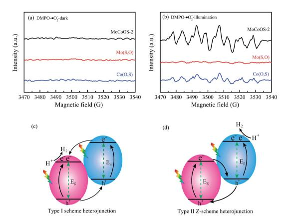
Fig. 14 EPR spectra of (a) DMPO-'O and (b) DMPO-'O<sub>2</sub>- for Mo(S,O), Co(O,S), and MoCoOS catalysts under darkness and illumination for 10 min. (c and d) The two types of heterojunction.
