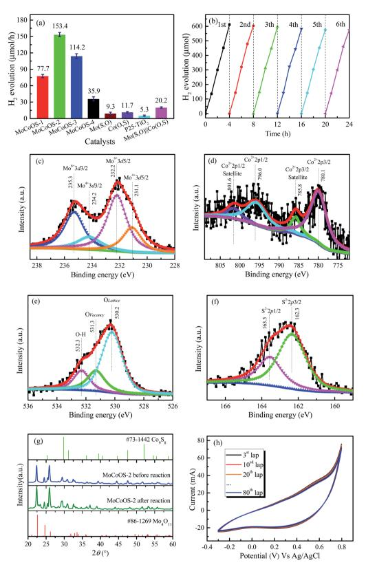
Fig. 7 (a) Hydrogen production of MoCoOS, Mo(S,O), Co(O,S), Mo(S,O)||Co(O,S) and P25-TiO $_2$  catalysts. (b) Recycling hydrogen production reaction performance of MoCoOS-2. (c-f) XPS spectra of MoCoOS-2 after the hydrogen evolution reaction. (g) XRD patterns of MoCoOS-2 before and after the hydrogen evolution reaction. (h) Cyclic voltammetry of MoCoOS-2 for 80 cycles.
