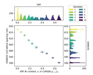
Fig. 3 Mean 110 lattice spacing as a function of the mean Br content determined from GIWAXS and XRF, respectively. Error bars represents  $\pm 1$  standard deviation of the mean. Histograms of all measured spots for the 10 samples are shown on top for the Br content from XRF and to the right for 110 lattice spacing from GIWAXS.
