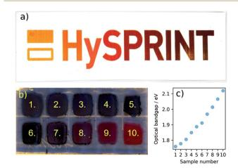
Fig. 1 (a) Logotype printed on paper with the different halide ratios of  $CsPb(Br_x|_{1-x})_{3,r}$  from the left to the right. (b) Combinatorial library of  $CsPb(Br_x|_{1-x})_3$  printed on quartz glass with ten samples from the top left to the bottom right labeled 1 to 10. (c) Optical bandgap of the ten samples from the combinatorial library in (b) determined from UV/vis transmission.
