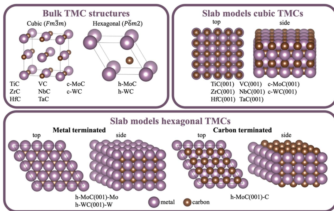
Fig. 1 Bulk and slab models used in the present work. The studied systems belonging to each bulk or slab model are indicated below the drawing.
