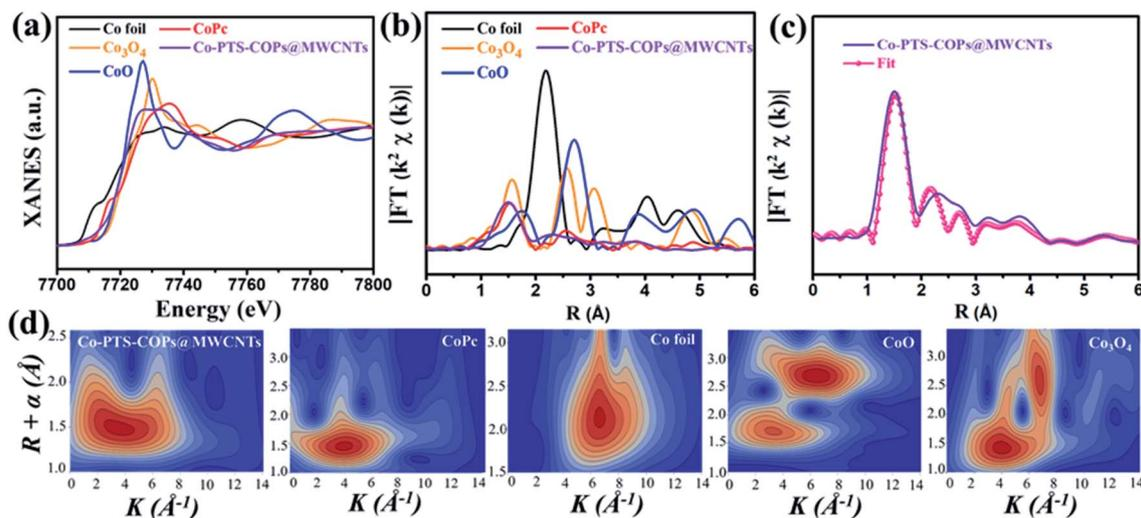
Fig. 3 (a) Co K edge XANES spectra and (b) Fourier-transformed EXAFS (FT-EXAFS) spectra of the Co-PTS-COPs@MWCNTs and standard samples (Co foil, CoO, Co<sub>3</sub>O<sub>4</sub> and CoPc), (c) FT-EXAFS fitting result of Co-PTS-COPs@MWCNTs in R space and (d) WT for the k<sup>3</sup>-weighted EXAFS signals.
