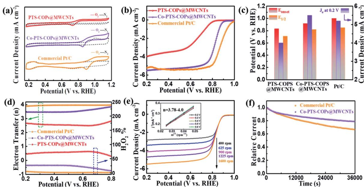
Fig. 4 (a) CV and (b) LSV curves, (c) *E*<sub>1/2</sub>, *E*<sub>onset</sub> and *J*<sub>d</sub>, and (d) H<sub>2</sub>O<sub>2</sub> yields and electron transfer number of Co-PTS-COPs@MWCNTs, PTS-COPs@MWCNTs and Pt/C. (e) LSV curves of Co-PTS-COPs@MWCNTs at different rotation speeds. Inset: the corresponding K–L plots and electron transfer number. (f) Chronoamperometric response of Co-PTS-COPs@MWCNTs and Pt/C.
