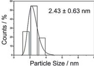
Fig. 8 Particle size distributions (PSD) in D-Co/SiO<sub>2</sub> catalysts, showing mainly small particles. The PSD show counts vs. particle size with a peak at about 2.4 nm.
