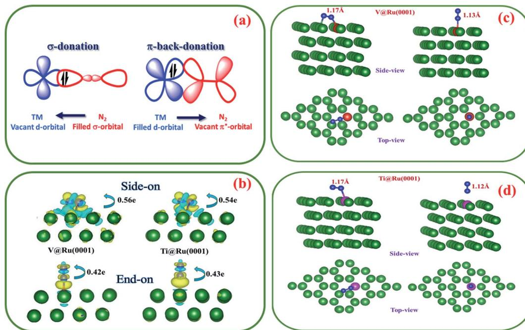
Fig. 4 (a) Schematic demonstration of N<sub>2</sub> bonding to a transition metal (TM). (b) The charge density difference of N<sub>2</sub> adsorbed on V@Ru(0001) and Ti@Ru(0001) in side-on and end-on configurations with the isosurface value set to 0.001 e Å<sup>-1</sup>; the yellow and cyan depict positive and negative charges, respectively. (c and d) The side-on and end-on binding of N<sub>2</sub> on V@Ru(0001) and Ti@Ru(0001), respectively.
