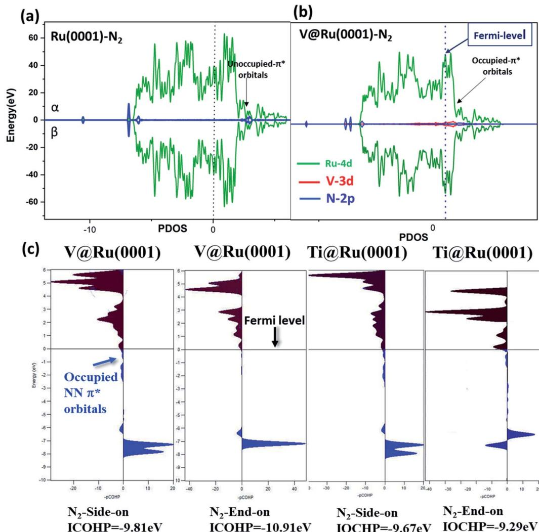
Fig. 5 Partial density of states (PDOS) for (a) nitrogen adsorbed on pure Ru(0001), (b) V@Ru(0001) (c) projected crystal orbital Hamiltonian population (pCOHP) for N<sub>2</sub> adsorption on V@Ru(0001) and Ti@Ru(0001) in side-on and end-on configurations.
