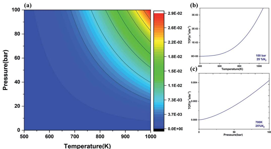
Fig. 8 (a) Contour plot depicting the turnover frequency (TOF) for the formation of  $\text{NH}_3$  over the V@Ru(0001) catalyst at various temperatures and pressures with 25% and 75% partial pressures of nitrogen and hydrogen, respectively; (b) graph depicting the variation of temperature with TOF at 100 bar pressure; (c) graph showing the variation of pressure with TOF at 700 K temperature for the V@Ru(0001) catalyst.
