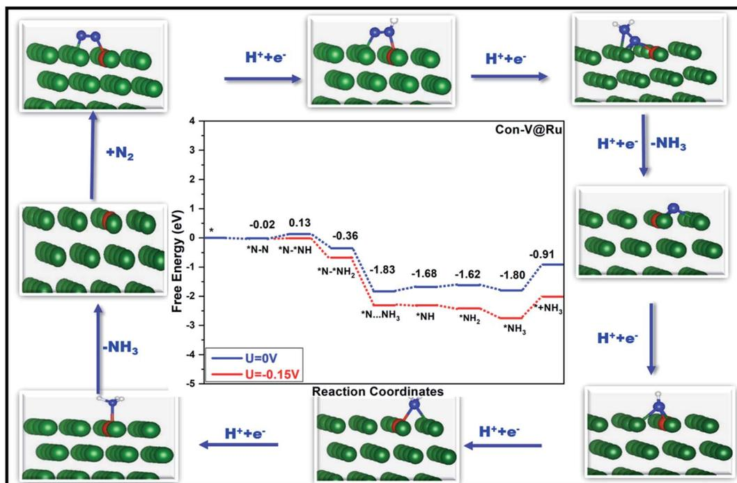
Fig. 6 Free-energy diagram for N<sub>2</sub> reduction via a consecutive mechanism at different applied potentials along with the corresponding structures of the intermediates involved in the reduction process. Green, red, blue and white balls represent Ru, V, N and H atoms, respectively.
