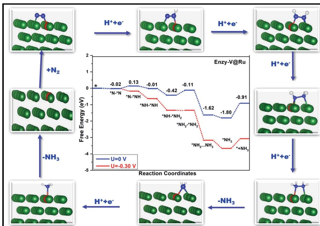
Fig. 7 Free-energy diagram for N<sub>2</sub> reduction via an enzymatic mechanism at different applied potentials along with the corresponding structures of the intermediates involved in the reduction process.
