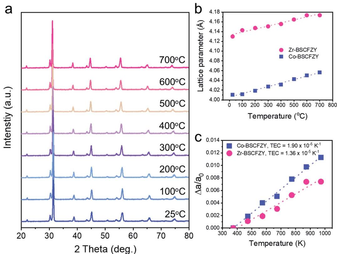
Fig. 3 (a) High-temperature X-ray diffraction (XRD) profile of  $\text{Ba}_{0.5}\text{Sr}_{0.5}\text{Co}_{0.6}\text{Fe}_{0.2}\text{Zr}_{0.1}\text{Y}_{0.1}\text{O}_{3-\delta}$  (BSCFZY), (b) lattice parameter expansion of the Zr-rich BSCFZY phase (Zr-BSCFZY) and Co-rich BSCFZY (Co-BSCFZY) phase as a function of the temperature, and (c) temperature-dependence of  $\Delta a/a_0$ .
