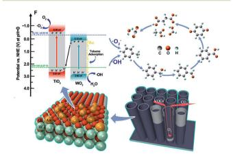
Scheme 1 Schematic mechanism for gaseous toluene degradation over the SAu-W/T.
