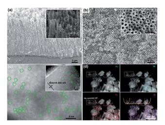
Fig. 1 (a) and (b) FE-SEM image of  $^{S}$ Au-W/T, (c) HAADF-TEM image of  $^{S}$ Au-W/T. Single Au sites are highlighted by green circles. (d) Elemental mappings of the selective HAADF-TEM image of  $^{S}$ Au-T/W. The elemental mappings illustrate the spatial distribution of Au (green), W (blue), and Ti (red), respectively.
