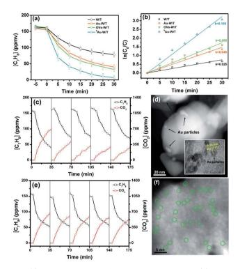
Fig. 6 (a) Photodegradation of toluene by samples and (b) pseudo first-order kinetic curve. (c) Recycle tests and (d) HAADF-TEM image of Au-W/T after the recycle; the insert is the TEM image of Au-W/T. (e) Recycle tests and (f) HAADF-TEM image of SAu-W/T after the recycle.
