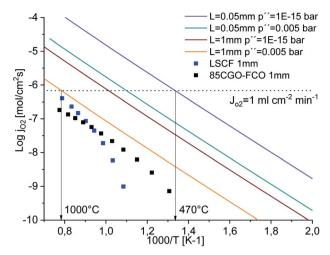
Fig. 26 The modelling of best-case performance of CGO20 for L=0.05 and 1 mm,  $p{\rm O''}_2=0.005$  and 10–15 bar, dashed line represents oxygen flux of 1 ml cm $^{-2}$  min $^{-1}$  as well as experimental data of LSCF and CGO–FCO 1 mm thick pellets.
