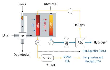
Fig. 25 OTM- SMR high-level process schematic.
