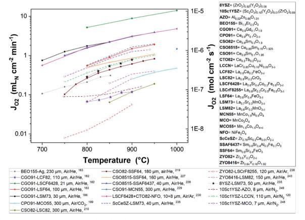
Fig. 8 Oxygen permeation flux of various thin ( $L \le 300~\mu m$ ) planar dual-phase OTMs as a function of the temperature.
