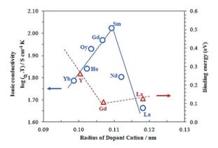
Fig. 7 Dependence of the ionic conductivity on ionic radius of  $M^{3+}$  for  $(CeO_2)_{0.8}(M_2O_3)_{0.2}$  systems at 800 °C. Reproduced with permission.<sup>89</sup> Copyright 2003, Elsevier.
