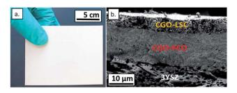
Fig. 12 Post-sintered picture (a) and SEM image of a fractured crosssection (b) of a planar dual-phase membrane component made from  $Ce_{0.8}Gd_{0.2}O_{2-\delta}-FeCo_2O_4$ . The post-sintered picture of the membrane was taken on the 3YSZ porous support side.
