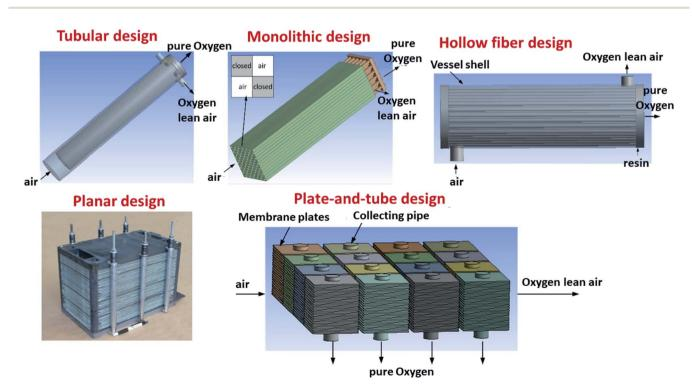
Fig. 11 Different design configurations for OTM modules.
