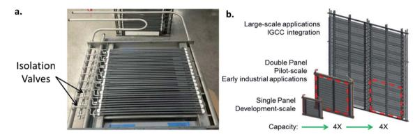
Fig. 19 Picture of (a) a single OTM unit panel array and (b) scaling panel size concept for large-scale applications.<sup>385</sup>
