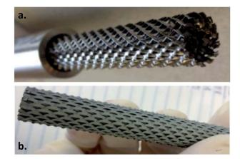
Fig. 20 Picture of (a) the components of the primary reformer (tube and catalysts support) and (b) catalyst-coated spiral metal monolith.389
