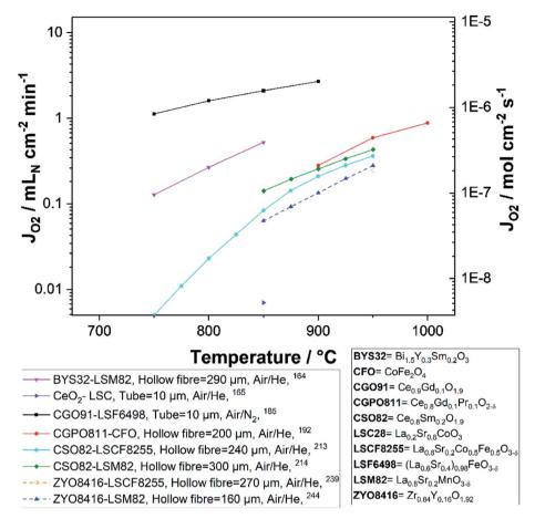
Oxygen permeation flux of various thin ( $L \le 300 \mu m$ ) tubular and hollow fiber dual-phase OTMs as a function of the temperature.
