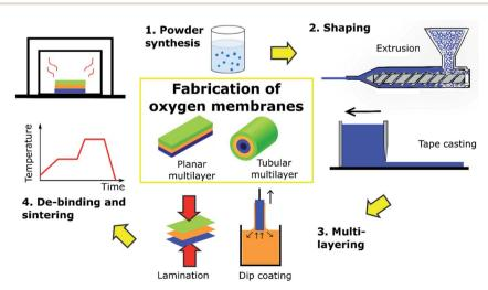
Fig. 13 Typical core steps in processing of planar and tubular multilayer dual-phase OTMs.
