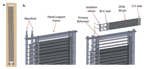
Fig. 18 Arrangement of the (a) M-pin assembly and (b) OTM unit panel arrays.<sup>389</sup>
