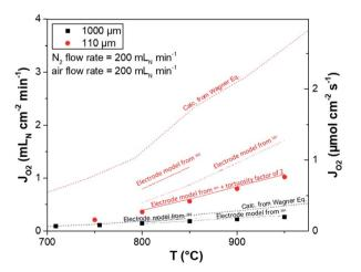
Fig. 28 Experimental (symbols) and theoretical (lines) oxygen permeation fluxes through 10Sc1YSZ-LCCN membranes coated with a 8YSZ-LSM (50-50 vol%) catalyst layer on both sides as a function of the temperature. The experiment was performed in air/N<sub>2</sub> atmosphere
