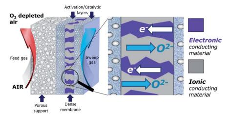
Schematic draw of an asymmetric dual-phase membrane.
