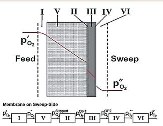
Fig. 1 Model of resistances representing the steps of the oxygen permeation through asymmetric membranes. Reproduced with permission.<sup>7</sup> Copyright 2014, Elsevier.
