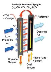
Fig. 17 OTM combined reformer for IGCC power systems concept developed by Praxair, Inc.252
