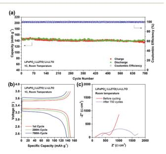
Fig. 8 The overall SSB cycling performance. (a) Cycling performance of LiFePO<sub>4</sub>|LLZTO|Li-LLTO at a rate of 1C at room temperature. (b) Charge and discharge curves for the  $1^{\rm st}$ ,  $200^{\rm th}$ , and  $700^{\rm th}$  cycles at 1C. (c) EIS curves of the fresh cell and cycled cell for the LiFePO<sub>4</sub>-|LLZTO|Li-LLTO SSB.
