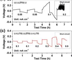
Fig. 4 (a) EIS curves for Li symmetric cells with different Li-LLTO compositions. (b) CCD for the pure Li in the Li symmetric cell. (c) CCD for the Li-LLTO composite in the Li symmetric cell.
