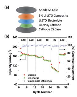
Fig. 7 The overall SSB cycling performance. (a) Assembly of the solidstate lithium batteries. (b) Performance of the LiFePO<sub>4</sub>|LLZTO|Li-LLTO solid-state cells at different charge—discharge rates.
