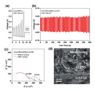
Fig. 5 (a) Li plating and stripping performance of the Li|LLZTO|Li symmetric cell with a current density of 0.1 mA cm<sup>-2</sup> at room temperature. (b) Li plating and stripping performance of the Li-LLTO|LLZTO|Li-LLTO symmetric cell at a current density of 0.1 mA cm<sup>-2</sup> at room temperature. (c) EIS of Li-LLTO|LLZTO|Li-LLTO before/ after cycling, and (d) SEM image of Li-LLTO|LLZTO|Li-LLTO after cycling
