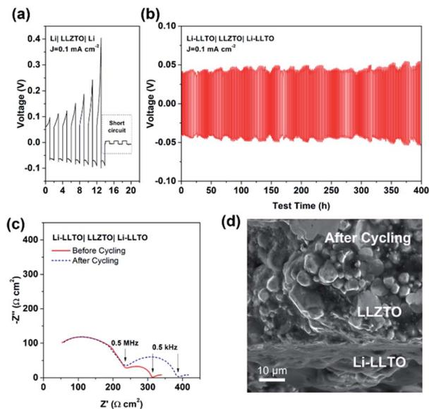
Fig. 5 (a) Li plating and stripping performance of the Li|LLZTO|Li symmetric cell with a current density of  $0.1 \text{ mA cm}^{-2}$  at room temperature. (b) Li plating and stripping performance of the Li-LLTO|LLZTO|Li-LLTO symmetric cell at a current density of  $0.1 \text{ mA cm}^{-2}$  at room temperature. (c) EIS of Li-LLTO|LLZTO|Li-LLTO before/after cycling, and (d) SEM image of Li-LLTO|LLZTO|Li-LLTO after cycling.
