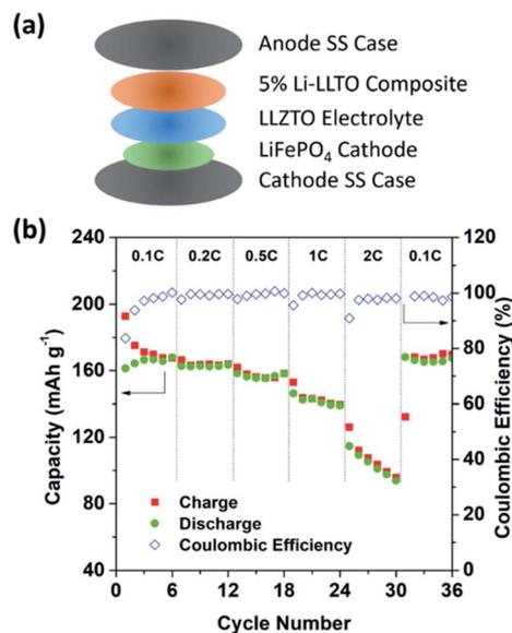
Fig. 7 The overall SSB cycling performance. (a) Assembly of the solid-state lithium batteries. (b) Performance of the  $\text{LiFePO}_4$ |LLZTO|Li-LLTO solid-state cells at different charge–discharge rates.
