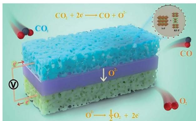
Scheme 1 Schematic illustration of the cell configurations of SOECs for CO<sub>2</sub> electrolysis.
