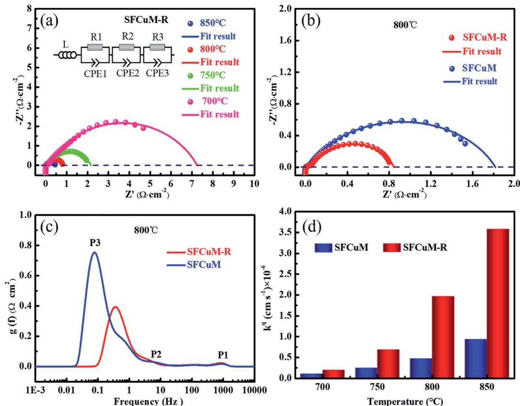
Fig. 7 (a) EIS of LSGM electrolyte-supported symmetrical cells with the configuration SFCuM-R/LDC/LSGM/LDC/SFCuM-R under a 1 : 1 CO<sub>2</sub>-CO<sub>2</sub> atmosphere at different operating temperatures; (b) comparison of the EIS spectra using different electrodes at 800 °C; (c) assessment of the DRT spectrum at 800 °C; (d) calculated  $k^q$  of the different electrodes.
