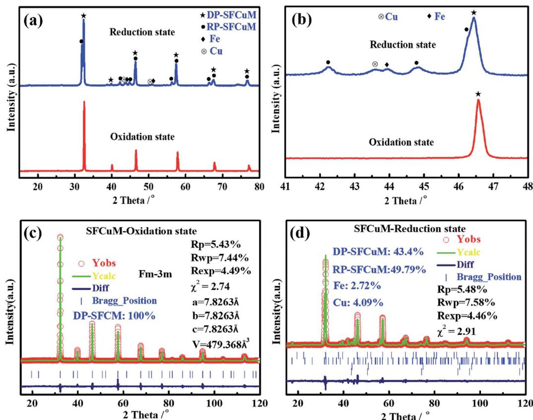
Fig. 1 (a) As-synthesized and reduced  $\text{Sr}_2\text{Fe}_{1.25}\text{Cu}_{0.25}\text{Mo}_{0.5}\text{O}_{6-\sigma}$  (SFCuM) powders, (b) magnification of (a), and (c) and (d) Rietveld refinement performed for the as-synthesized and reduced SFCuM powders, respectively.
