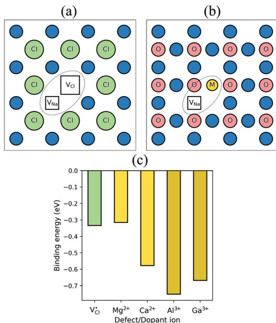
Fig. 4 Defect clustering in Na<sub>3</sub>OCl (a) undoped structure with sodium and chloride vacancies; (b) doped structures with a sodium vacancy and a dopant ion. (c) Binding energies for pair clusters.
