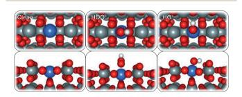
Fig. 1 Top (top) and side (bottom) view of SnO<sub>2</sub>-supported single metal atom surfaces with adsorbed reaction intermediates (atoms in grey = Sn, red = oxygen, white = hydrogen, blue = Sn, Ru, V, Co, Pd, Pt, Ni, Mo, Ir, Cr, Mn, Fe, W, Ti, Sb, Nb, or Ta).
