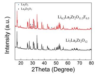
Fig. 1 XRD patterns obtained for  $\text{Li}_{7-x}\text{La}_3\text{Zr}_2\text{O}_{12-x}\text{F}_x$ : x=0 and 0.5 showing significant impurities for x=0.5 and no change in the level of tetragonal distortion; LiF was used as the fluorine source.
