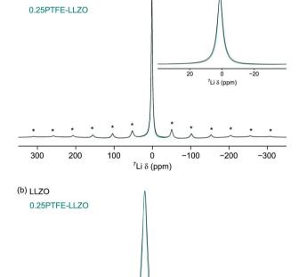
Fig. 7 (a) <sup>7</sup>Li and (b) <sup>6</sup>Li MAS NMR spectra obtained for LLZOF and LLZO. Spectra are the result of (a) 16, 32 and (b) 200 transients with a recycle interval of 90 s. A MAS rate of 10 kHz was used and spinning sidebands are denoted by \*. In (a) an expansion of the central transition is also shown.
