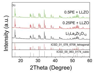
Fig. 2 XRD patterns obtained for samples of Li<sub>7</sub>La<sub>3</sub>Zr<sub>2</sub>O<sub>12</sub> mixed with (a) PTFE and (b) PE at 400  $^{\circ}$ C in dry N<sub>2</sub>, indicating a reduction in tetragonal distortion for the reaction with PTFE and no change upon reaction with PE
