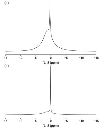
Fig. 9  $\,^{7}$ Li MAS NMR spectra of (a) 0.75PVC:LLZO and (b) 1.0PVC:LLZO. Each spectrum is the result of averaging 64 transients with a recycle interval of 6 s. A MAS rate of 10 kHz was used.
