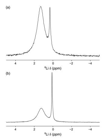
Fig. 10 <sup>6</sup>Li MAS NMR spectra of (a) 0.75PVC:LLZO and (b) 1.0PVC:LLZO. Each spectrum is the result of averaging 200 transients with a recycle interval of 8 s. A MAS rate of 10 kHz was used.
