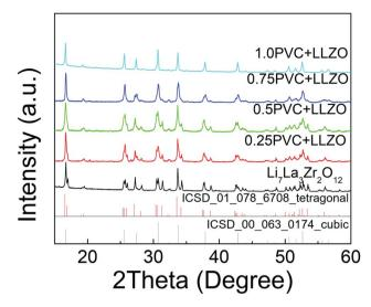
Fig. 4 XRD patterns obtained for samples of Li<sub>7</sub>La<sub>3</sub>Zr<sub>2</sub>O<sub>12</sub> mixed with PVC showing formation of a cubic cell for higher Cl levels.
