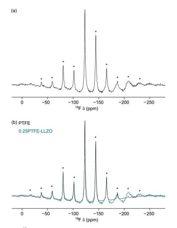
Fig. 8  $^{19}$ F MAS NMR spectra obtained for (a) LLZOF and (b) PTFE. In (b), the spectrum for LLZOF is also shown for comparison. Spectra are the result of (a) 320 and (b) 16 transients with a recycle interval of 10 s. A MAS rate of 10 kHz was used and spinning sidebands are denoted by \*.
