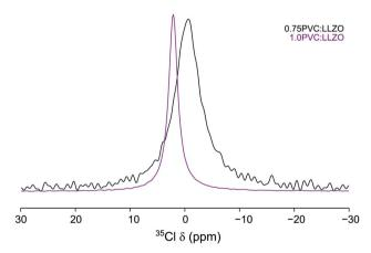
Fig. 11 <sup>35</sup>Cl MAS NMR spectra of 0.75PVC:LLZO and 1.0PVC:LLZO Each spectrum is the result of averaging 1600 transients with a recycle interval of 0.4 s. A MAS rate of 10 kHz was used
