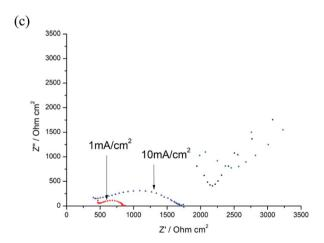
Fig. 14 (a) Constant current cycling testing of Li/LLAZO(PTFE)/Li cell from 1 mA cm<sup>-2</sup> to 10 mA cm<sup>-2</sup> (b) EIS of the cell before and after cycling. (c) EIS of the cell after 1 mA  $\rm cm^{-2}$  and 10 mA  $\rm cm^{-2}$  cycling
