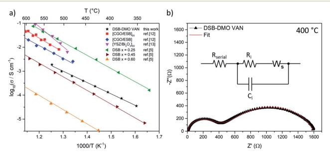
Fig. 3 (a) Arrhenius plot of DSB-DMO VAN film in air displaying high ionic conductivity as compared to the literature results for superlattices<sup>12,13</sup> and bulk powder DSB<sup>5</sup> (b) typical Nyquist plot at 400 °C. Inset; the Randles model used to fit the data, where  $R_i/C_i$  models the ionic conductivity of DSB,  $W_s$  the FLW response, and  $R_{serial}$  the internal resistances of the EIS setup.
