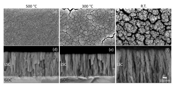
Fig. 1 Typical plan-view SEM images of as-grown LSC films deposited at (a) 500 °C, (b) 300 °C, and (c) room temperature (R.T.). The film deposited at R.T. exhibits the highest porosity among the samples. The corresponding cross-sectional SEM images are shown in (d–f). The characteristic nanostructures vary widely depending on deposition temperature. The scale bar shown in image (f) corresponds to the scale of all images.
