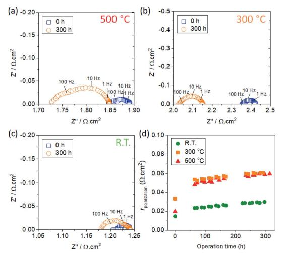
Fig. 8 Impedance spectra for LSC thin films deposited at (a)  $500 \,^{\circ}$ C, (b)  $300 \,^{\circ}$ C, and (c) room temperature (R.T.). The data at t = 0 h and 300 h are depicted by square and circle symbols, respectively. The overall electrode resistance,  $r_{polarization}$ , is plotted versus operation time in (d). 500 °C: red triangles, 300 °C: orange squares, R.T.: green circles
