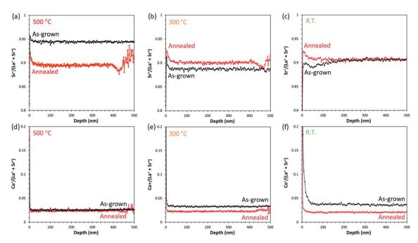
Fig. 6 Secondary ion ratios of  $Sr^+/(La^+ + Sr^+)$  (top row) and  $Co^+/(La^+ + Sr^+)$  (bottom row) derived from ToF-SIMS data for the as-grown and annealed LSC thin films prepared at 500 °C ((a) and (d)), 300 °C ((b) and (e)), and R.T. ((c) and (f)).
