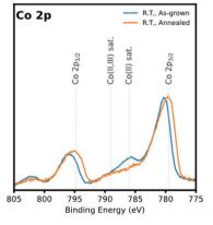
Fig. 5 X-ray photoelectron spectra of Co 2p of the LSC nanostructured films grown at 500 °C, 300 °C, and R.T. As-grown films and annealed films are depicted in blue and orange, respectively.
