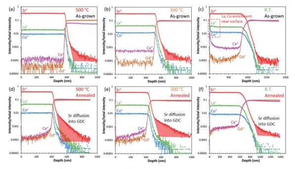
Fig. 7 SIMS depth profiles of LSC/GDC samples prepared at (a)  $500 \,^{\circ}$ C, (b)  $300 \,^{\circ}$ C, and (c) R.T., and annealed samples are shown respectively in (d), (e) and (f). Areas highlighted in red indicate regions of Sr diffusion into the GDC layer.
