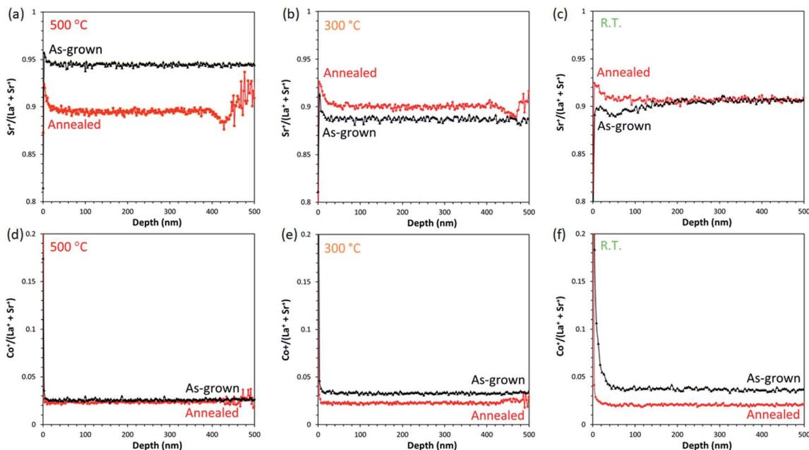
Fig. 6 Secondary ion ratios of Sr<sup>+</sup>/(La<sup>+</sup> + Sr<sup>+</sup>) (top row) and Co<sup>+</sup>/(La<sup>+</sup> + Sr<sup>+</sup>) (bottom row) derived from ToF-SIMS data for the as-grown and annealed LSC thin films prepared at 500 °C ((a) and (d)), 300 °C ((b) and (e)), and R.T. ((c) and (f)).
