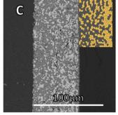
Fig. 1 Microstructure of the mixed cathodes from SEM images (a) thick cathode, (b) thin cathode, (c) gradient cathode.
