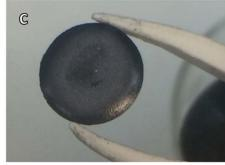
Fig. 2 Flatness and phase composition of a thick tape-cast LCO/LLZO layer after sintering at 1050 °C in air for 2 h; (a) white-light topography; (b) XRD pattern (c) picture of free-standing mixed cathode
