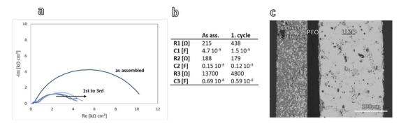
Fig. 3 (a): Impedance spectra at 80 °C of the model cell including a thick cathode as assembled and after cycling; (b): fit of the impedance data of the as assembled cell and after the first charge-discharge cycle; (c): cross-section of the model cell.
