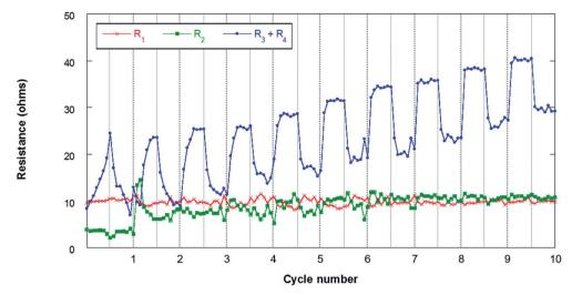
Evolution of the resistances during cycling for the  $Sn_4P_3/C//GDL$  cell. The lines connecting the data points are only a guide to the eye.
