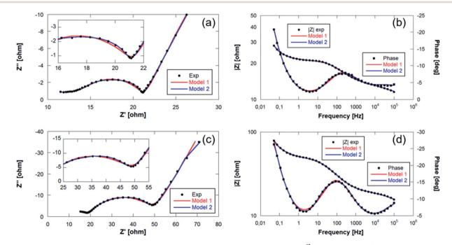
Fig. 10 Bode and Nyquist plots with fitting values collected at (a and b) final charge step of the  $1^{st}$  cycle and (c and d) start of the discharge of the  $6^{th}$  cycle of  $Sn_4P_3/C//GDL$  cell.
