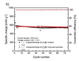
Fig. 3 Comparison of cycling behaviors of  $Sn_4P_3/C$  samples A and H at 100 mA  $g^{-1}$  at two different voltage windows of 1.5–0.005 V (a) and 1.5-0.05 V (b).
