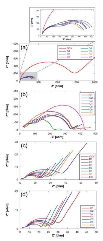
Fig. 8 Nyquist plots for (a and b) Na metal and (c and d) Sn<sub>4</sub>P<sub>3</sub>/C negative electrodes. C: charge; EC: end of charge; D: discharge; ED: end of discharge
