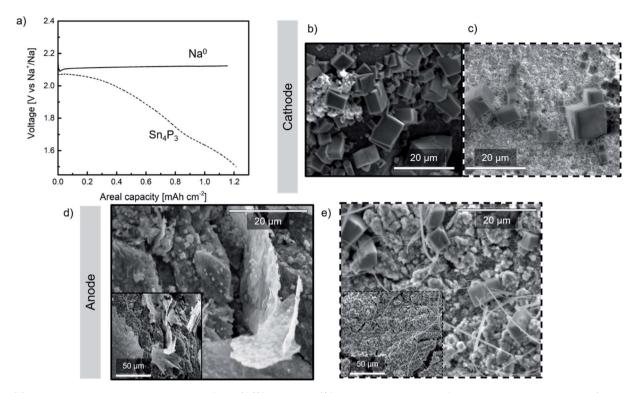
Fig. 5 (a) First discharge voltage profiles of the  $Sn_4P_3/C//GDL$  and Na//GDL cells; post mortem SEM images of both cathodes (b and c) and anodes (d and e). SEM images of the  $Sn_4P_3$  alloy are highlighted with a dash square.
