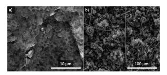
Fig. 4 SEM images of metallic Na (a) and  $Sn_4P_3/C$  (b) anodes after the chemical stability test.
