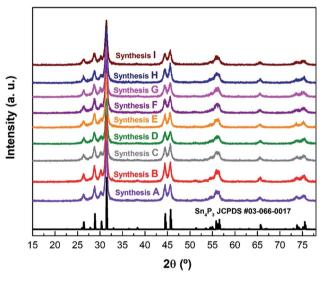
Fig. 1 The XRD patterns of the different syntheses of Sn<sub>4</sub>P<sub>3</sub>/C samples listed in Table 1 along with the reference pattern of Sn<sub>4</sub>P<sub>3</sub> (JCPDS #03-066-0017).
