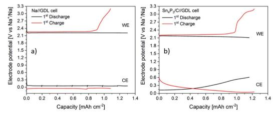
Fig. 7 Galvanostatic curves for each electrode of the Na//GDL (a) and  $Sn_4P_3/C//GDL$  cells (b) corresponding to the first discharge (black) and charge (red) curves during the EIS measurements. WE refers to the working electrode, i.e., the cathode and CE to the counter, i.e., the anode.
