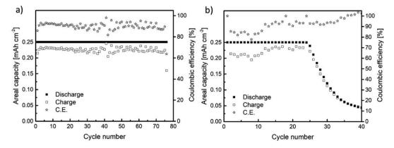
Fig. 6 Galvanostatic charge/discharge results for the cells assembled using (a) metallic Na (Na//GDL) and (b) Sn<sub>4</sub>P<sub>3</sub> (Sn<sub>4</sub>P<sub>3</sub>/C//GDL) negative electrodes.
