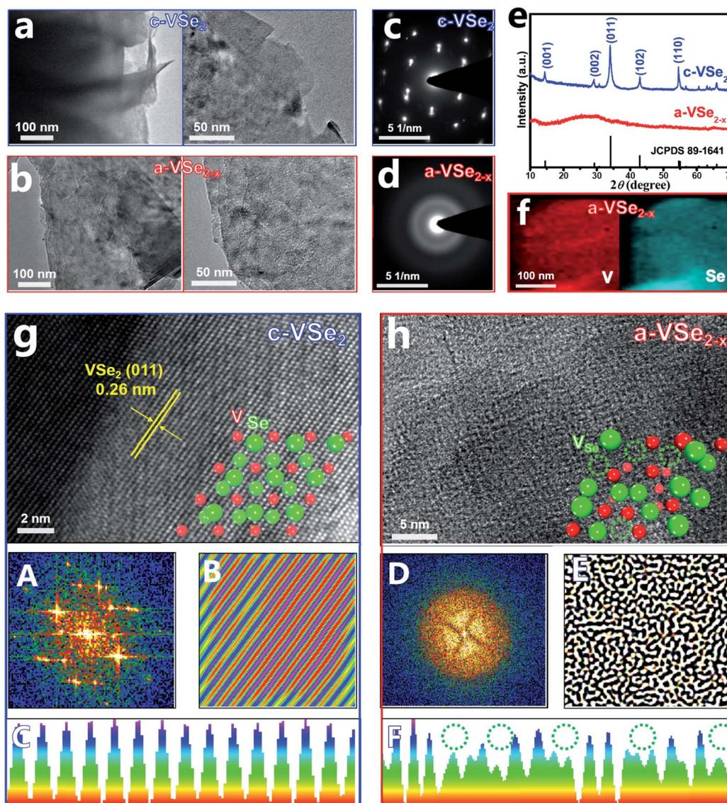
**Fig. 1** (a and b) TEM images of  $\text{c-VSe}_2$  and  $\text{a-VSe}_{2-x}$  at various magnifications. (c and d) SAED patterns of  $\text{c-VSe}_2$  and  $\text{a-VSe}_{2-x}$ . (e) XRD patterns of  $\text{c-VSe}_2$  and  $\text{a-VSe}_{2-x}$ . (f) Elemental mapping images of  $\text{a-VSe}_{2-x}$ . (g and h) HRTEM images of  $\text{c-VSe}_2$  and  $\text{a-VSe}_{2-x}$  (inset: atomic structure models) and corresponding FFT, IFFT and lattice line scanning analyses (panel A–F).
