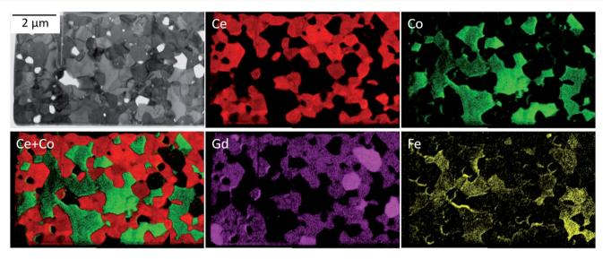
Fig. 2 Energy-filtered TEM (EFTEM) analysis identifying three main phases: Gd-doped ceria (red), Fe/Co-oxide (green) and the GdFeO<sub>3</sub>-based perovskite (bright magenta).
