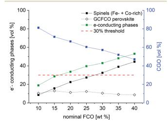
Fig. 5 Volume fraction of detected phases in the CGO-FCO composites sintered at 1200  $^{\circ}\text{C}$  for 5 h.
