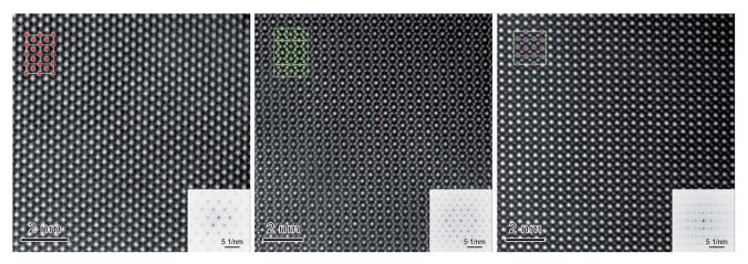
Fig. 3 High-resolution HAADF images of single grains of CGO (left), FCO (middle) and GCFCO (right) recorded along the [101], [101] and [110] zone axis, respectively. Upper left/lower right insets are the corresponding structural models/diffraction patterns measured in the TEM mode. Oxygen is not shown.
