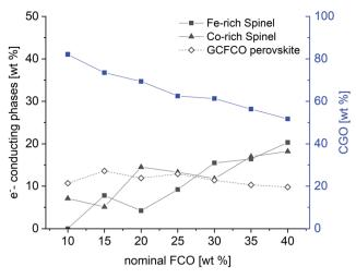
Fig. 4 Weight fraction of detected phases in the CGO-FCO composites sintered at  $1200\,^{\circ}\text{C}$  for 5 h according to Table 1.
