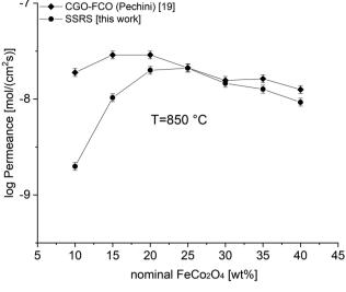
Fig. 9 Permeance of differently synthesized composites depending on the nominal FCO-content. Error bars represent  $\pm$  10% of the measured values
