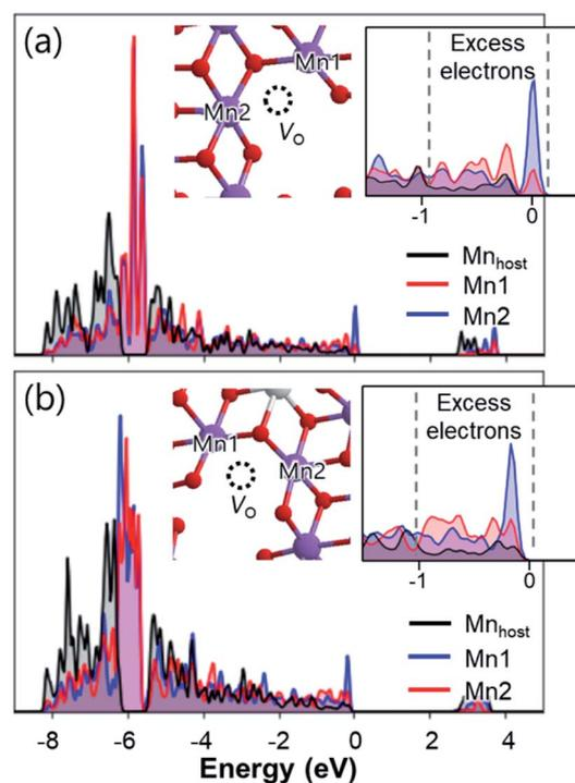
Fig. 6 Projected density of states of Mn atoms before ( $Mn_{host}$ ) and after (Mn1 and Mn2) the formation of O vacancies in (a)  $Na_2Mn_3O_7$  and (b)  $Na_{2.4}Al_{0.4}Mn_{2.6}O_7$ . Insets show O vacancy positions, reduced Mn atoms, and magnified density of states near excess electrons.
