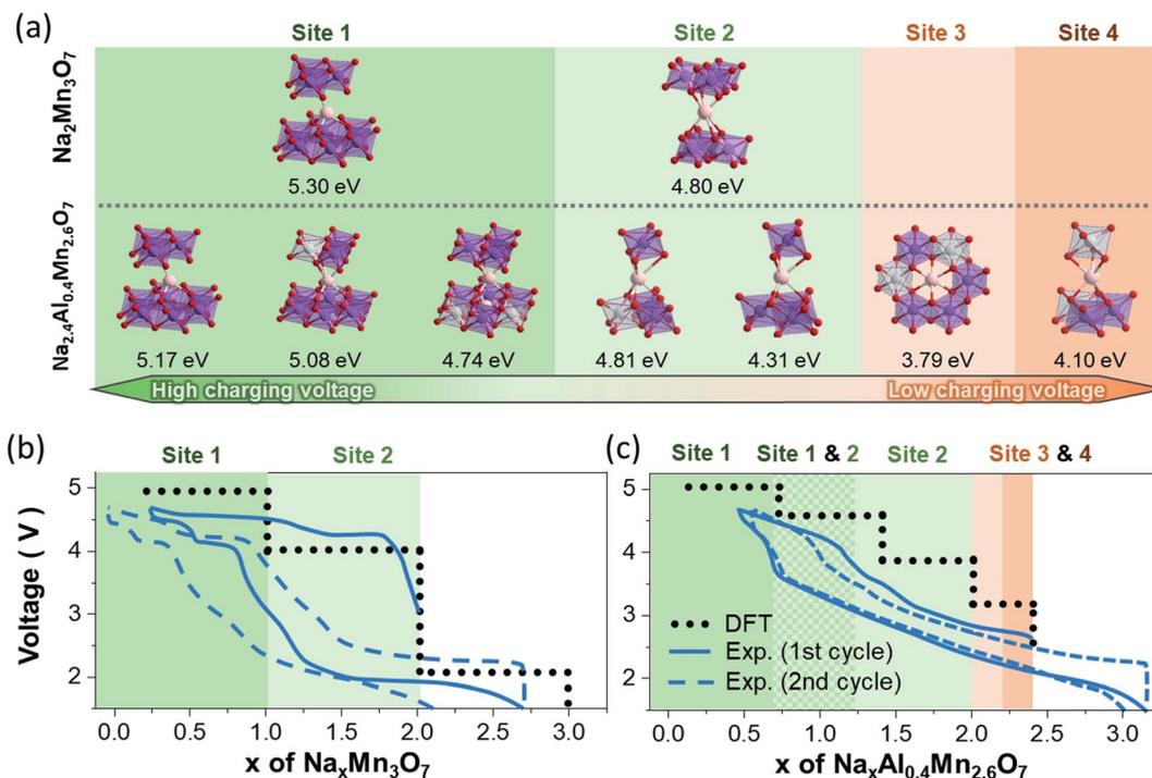
Fig. 4 (a) Local bonding environment of Na sites and their predicted Na vacancy formation energies in  $\text{Na}_x\text{Mn}_3\text{O}_7$  and  $\text{Na}_x\text{Al}_{0.4}\text{Mn}_{2.6}\text{O}_7$ . Theoretical and experimental voltage profiles of (b)  $\text{Na}_x\text{Mn}_3\text{O}_7$  and (c)  $\text{Na}_x\text{Al}_{0.4}\text{Mn}_{2.6}\text{O}_7$ . Electrochemically active Na sites for each Na content range are highlighted in differing colours.
