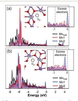
Fig. 6 Projected density of states of Mn atoms before (Mn $_{host}$ ) and after (Mn1 and Mn2) the formation of O vacancies in (a) Na $_2$ Mn $_3$ O $_7$  and (b) Na $_2$ .4Al $_0$ .4Mn $_2$ .6O $_7$ . Insets show O vacancy positions, reduced Mn atoms, and magnified density of states near excess electrons.
