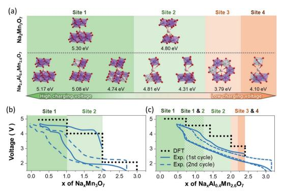
Fig. 4 (a) Local bonding environment of Na sites and their predicted Na vacancy formation energies in  $Na_xMn_3O_7$  and  $Na_xAl_{0.4}Mn_{2.6}O_7$ . Theoretical and experimental voltage profiles of (b)  $Na_xMn_3O_7$  and (c)  $Na_xAl_{0.4}Mn_{2.6}O_7$ . Electrochemically active Na sites for each Na content range are highlighted in differing colours.
