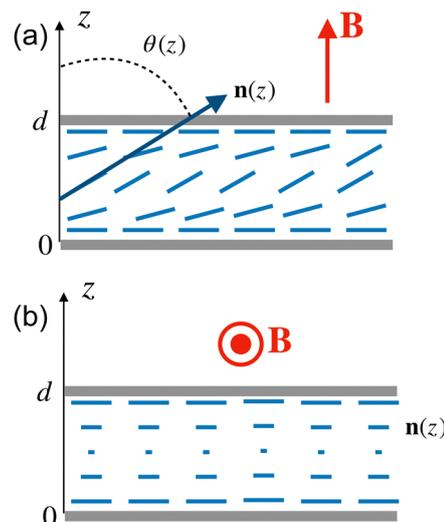
Fig. 2 Liquid crystal cells: (a) splay configuration with a magnetic field applied perpendicular to the substrate and the unperturbed director  $\mathbf{n}$ , and (b) twist configuration with a magnetic field applied parallel to the substrate and perpendicular to the director  $\mathbf{n}$ .
