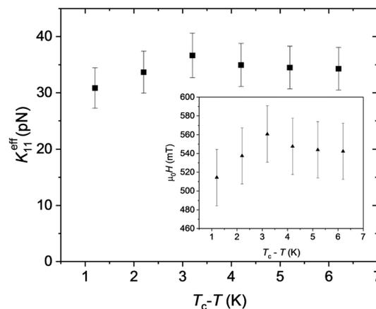
Fig. 11 Temperature dependence of the splay elastic constant measured in a 25 μm cell with polyimide rubbed substrates. The critical magnetic field  $\mu_0 H_c$  is given in the inset.
