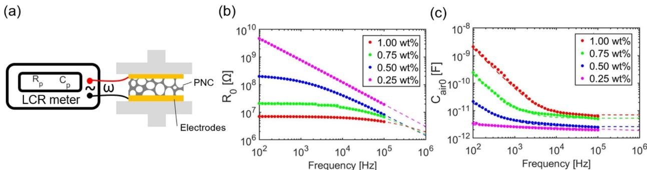
Fig. 3 (a) A schematic of the experimental setup for measuring the frequency response of PNC without and with applied pressure.  $R_p$  and  $C_p$  represent the resistance and capacitance measured by the LCR meter in the parallel mode. Frequency response of the (b) resistance and (c) capacitance of the PNC with different CNT doping ratios.  $R_0 = R_p$  and  $C_{\text{air0}} = C_p$ . Dashed curves are fitted based on eqn (2) and (3).
