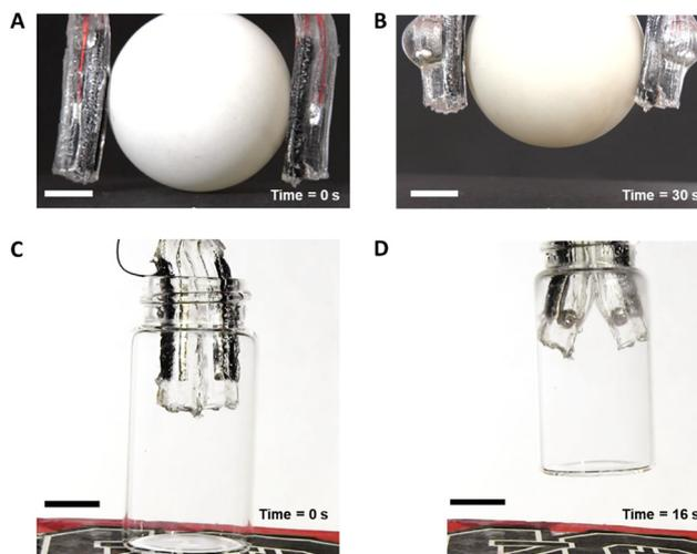
Fig. 4 Bubble actuator gripper. Photographs demonstrating the two modes of gripping: (A and B) inward curl gripping and (C and D) outward curl gripping. The grippers held the objects firmly after lifting them off the ground (B) a ball of 4 cm diameter and (D) a 20 ml glass vial in 30 s and 16 s respectively when a voltage input of 10 V is applied. The demonstrations can be found in ESI,† Videos S4 and S5. The scale bars represent 1 cm.
