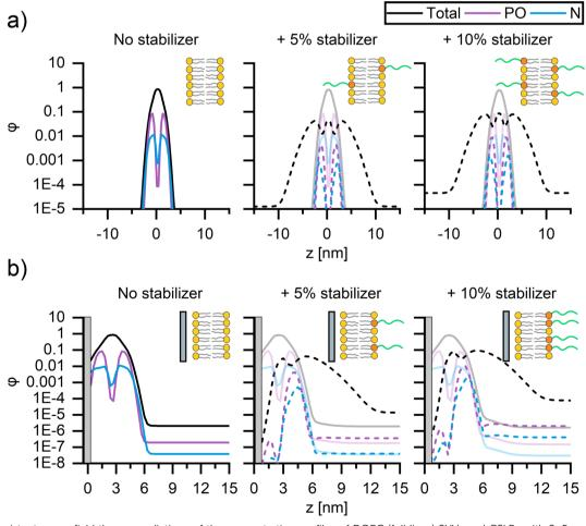
Fig. 4 Self-consistent mean-field theory predictions of the concentration profiles of DOPC (full lines) SUVs and CSLBs with 0, 5 mol% and 10 mol% DSPE-PEG<sub>2000</sub> (dotted lines). The average spatial composition profiles and corresponding schematic representations of (a) SUVs and (b) CSLBs composed of DOPC with 0 (left), 5 mol% (middle) and 10 mol% (right) DSPE-PEG<sub>2000</sub> stabilizer. The silica surface in b is represented by the grey region.
